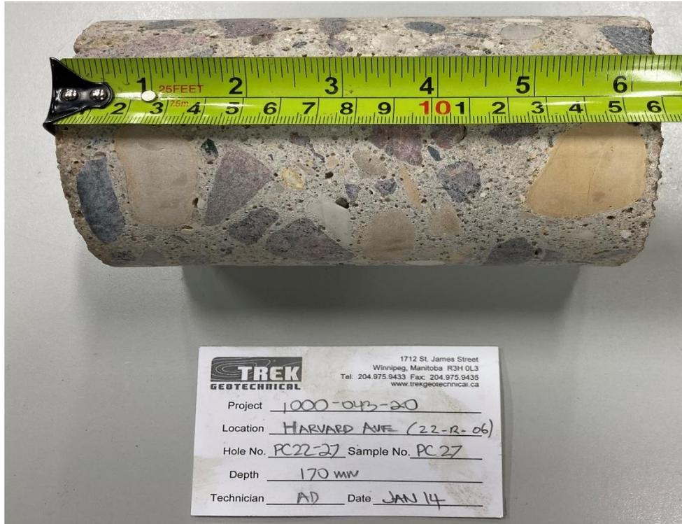
Photo 3: Pavement Core Sample at PC22-27
