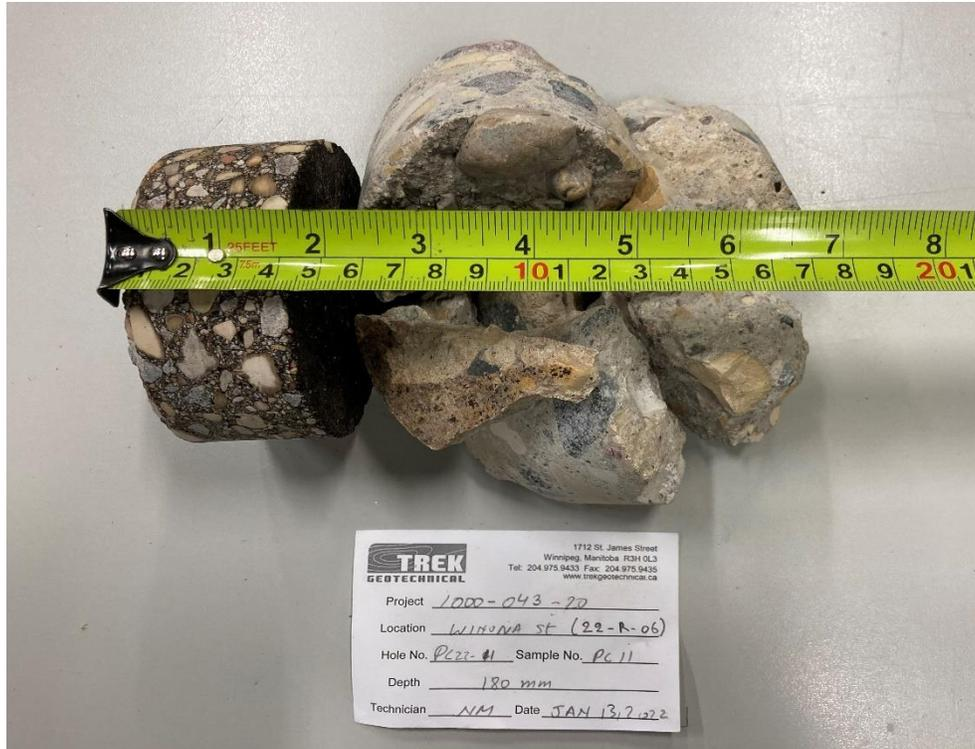
Photo 1: Pavement Core Sample at PC22-11
