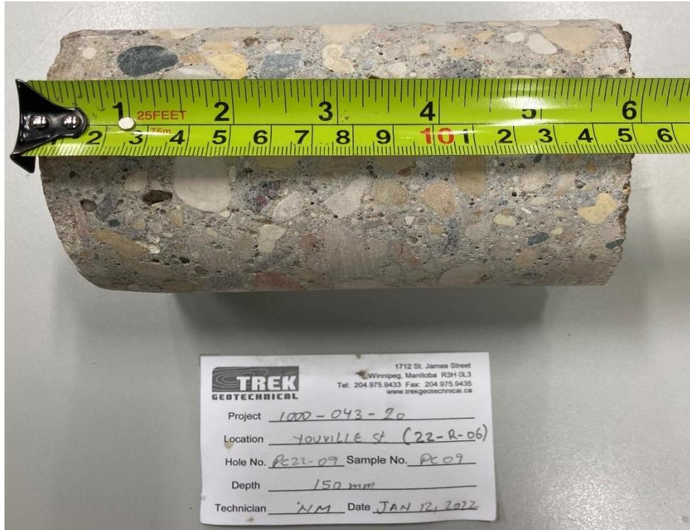
Photo 3: Pavement Core Sample at PC22-09
