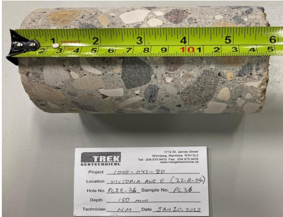
Photo 3: Pavement Core Sample at PC22-36
