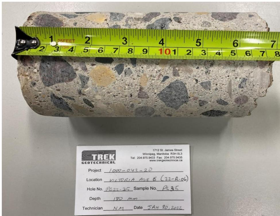
Photo 2: Pavement Core Sample at PC22-35
