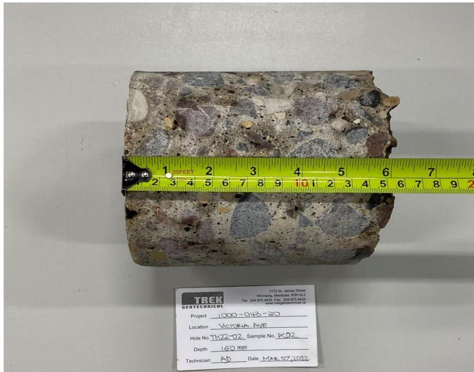
Photo 2: Pavement Core Sample at TH22-02
