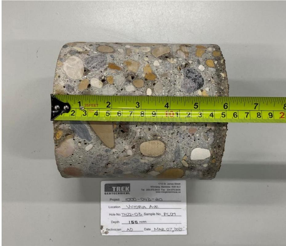
Photo 3: Pavement Core Sample at TH22-03
