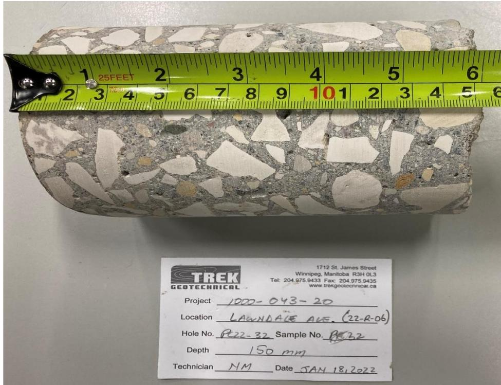
Photo 5: Pavement Core Sample at PC22-32
