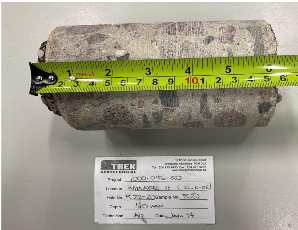
Photo 2: Pavement Core Sample at PC22-20
