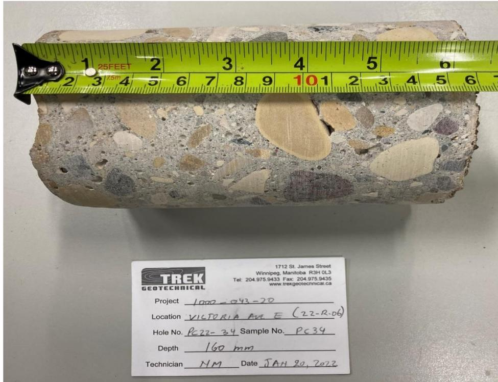
Photo 1: Pavement Core Sample at PC22-34
