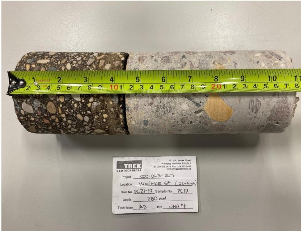
Photo 1: Pavement Core Sample at PC22-19
