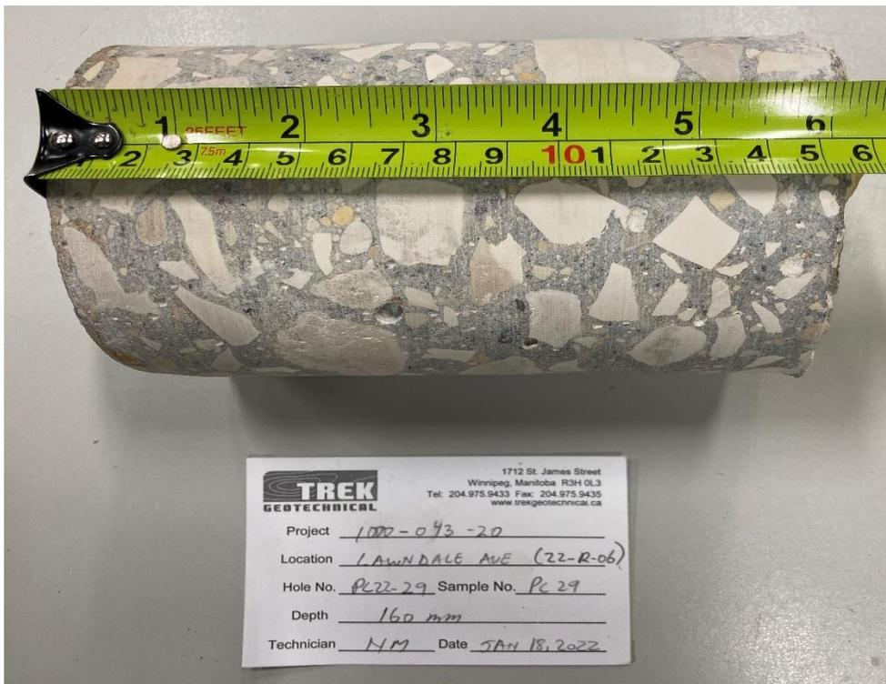
Photo 2: Pavement Core Sample at PC22-29
