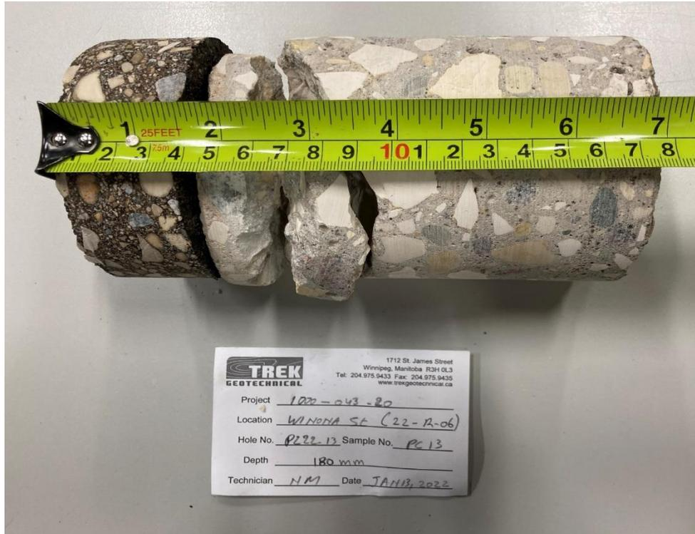
Photo 3: Pavement Core Sample at PC22-13
