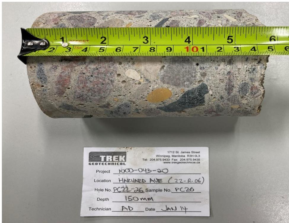
Photo 2: Pavement Core Sample at PC22-26
