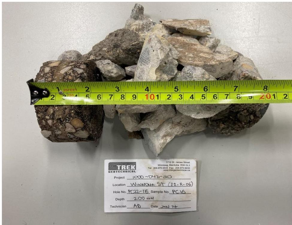
Photo 6: Pavement Core Sample at PC22-16
