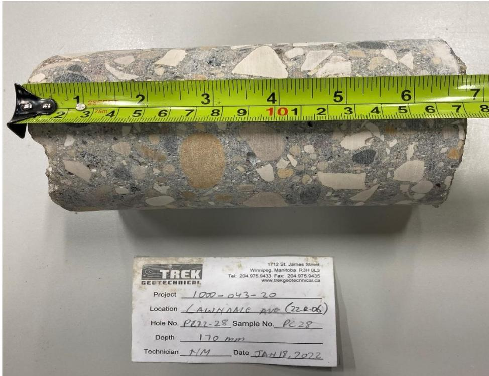
Photo 1: Pavement Core Sample at PC22-28
