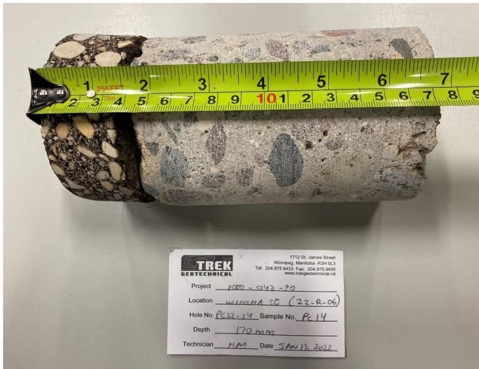
Photo 4: Pavement Core Sample at PC22-14
