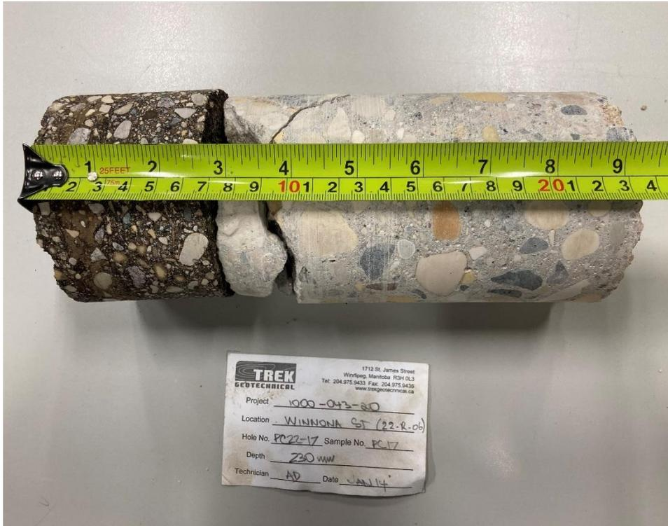
Photo 7: Pavement Core Sample at PC22-17
