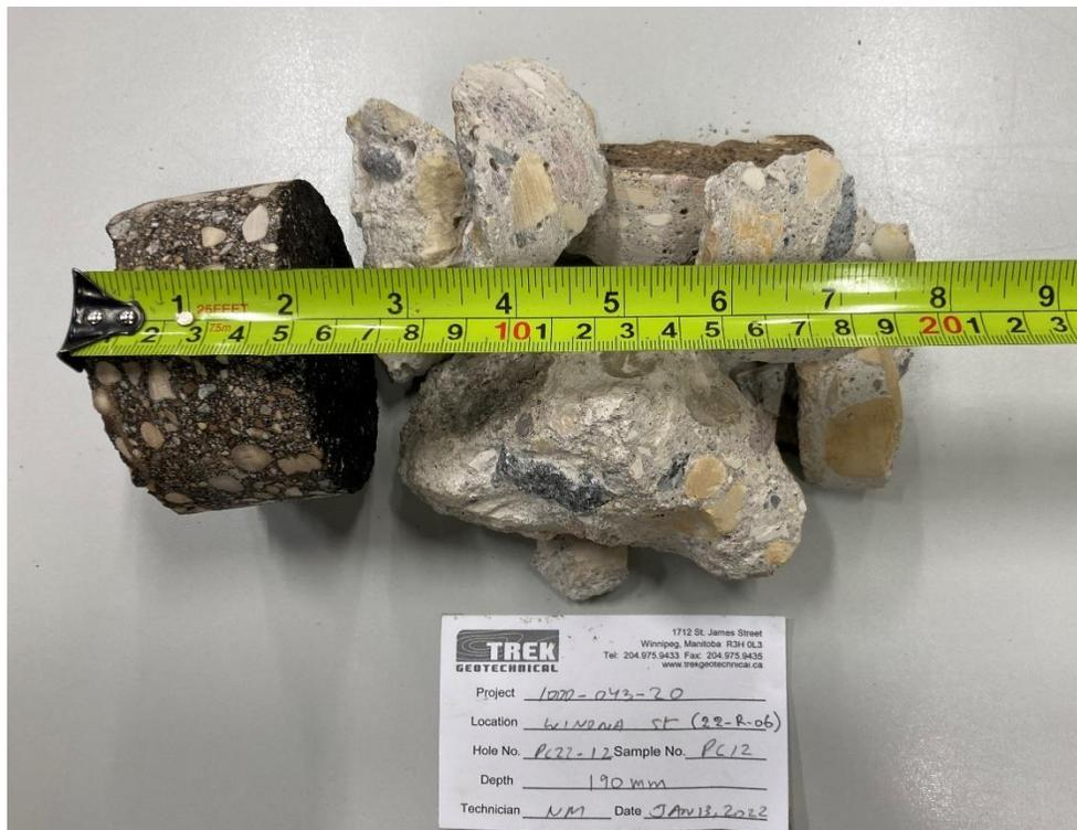
Photo 2: Pavement Core Sample at PC22-12
