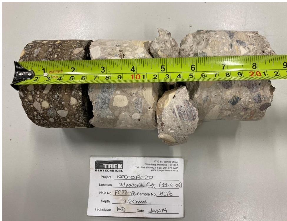
Photo 8: Pavement Core Sample at PC22-18
