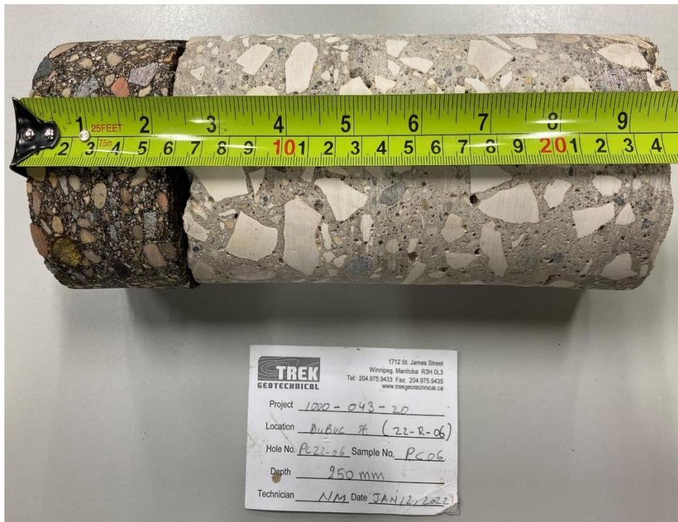
Photo 6: Pavement Core Sample at PC22-06
