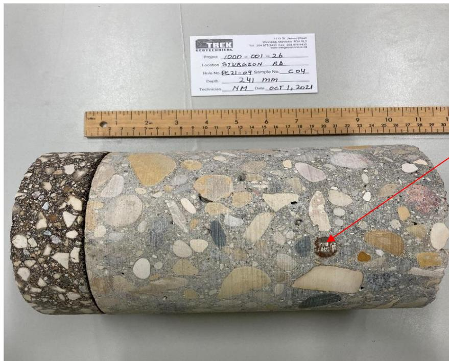
Photo 4: Pavement Core Sample at PC21-04
