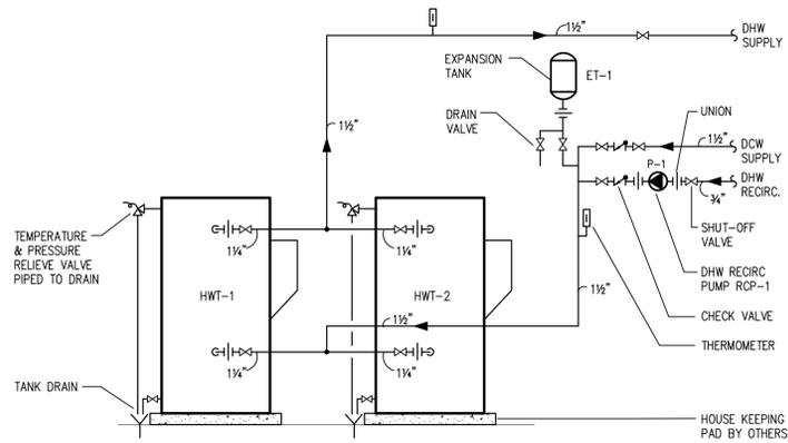
**ELECTRIC HOT WATER TANK DETAIL**
