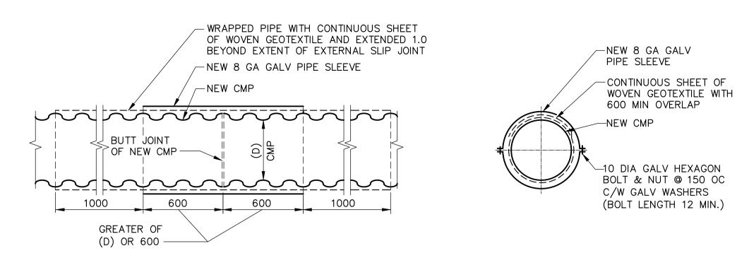
EXTERNAL SLIP JOINT DETAIL SCALE: N.T.S.
