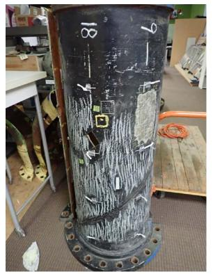
Photo 5. Paint Sample S-04 location (black piping system; RAS 2 HPO Reactor Inlet) from off-site pipe located at Testlabs International.
