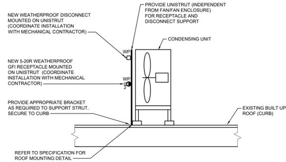
**1** TYPICAL ROOF RECEPTACLE AND DISCONNECT MOUNTING DETAIL
