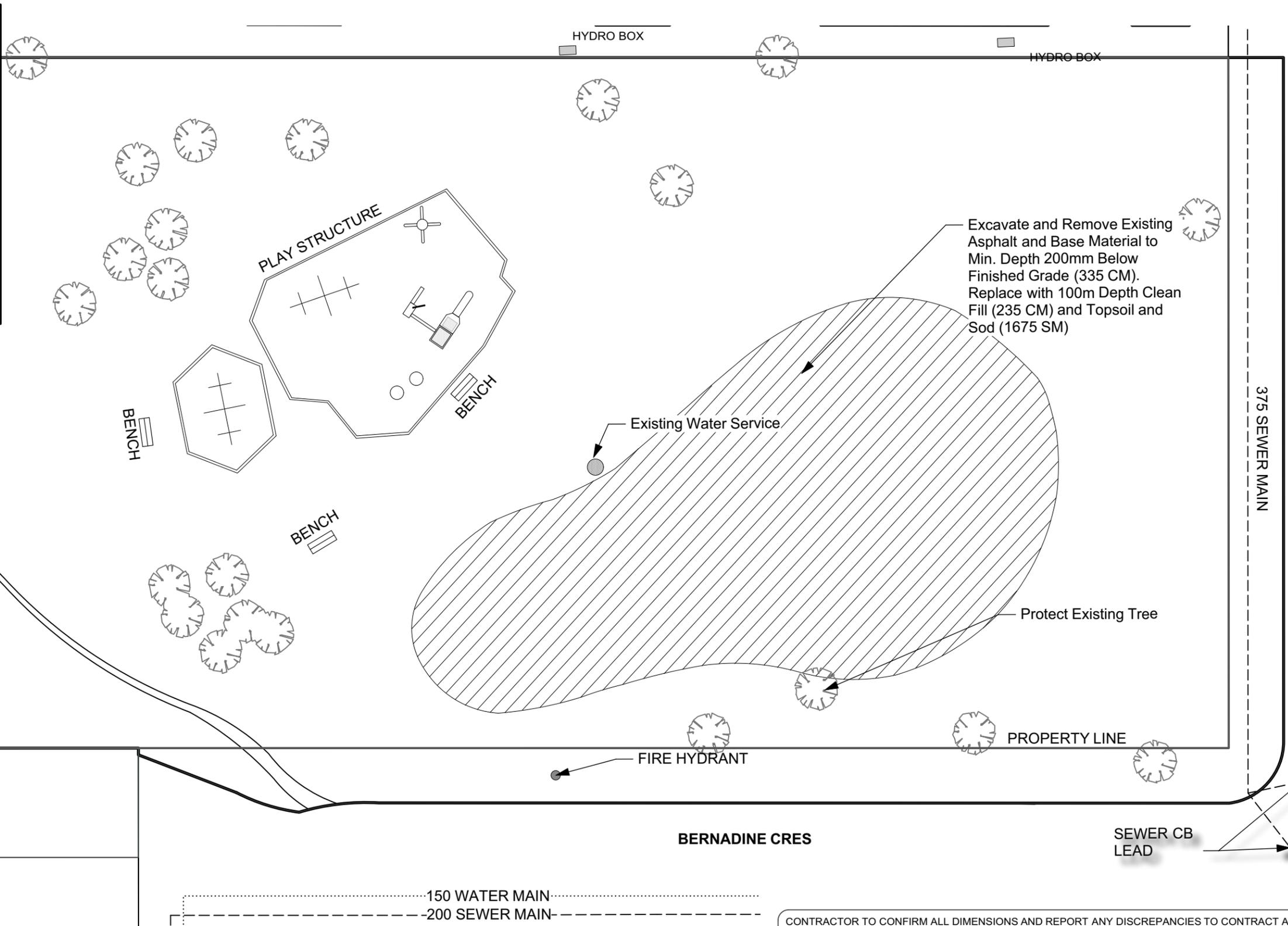
Excavate and Remove Existing Asphalt and Base Material to Min. Depth 200mm Below Finished Grade (335 CM). Replace with 100m Depth Clean Fill (235 CM) and Topsoil and Sod (1675 SM)
