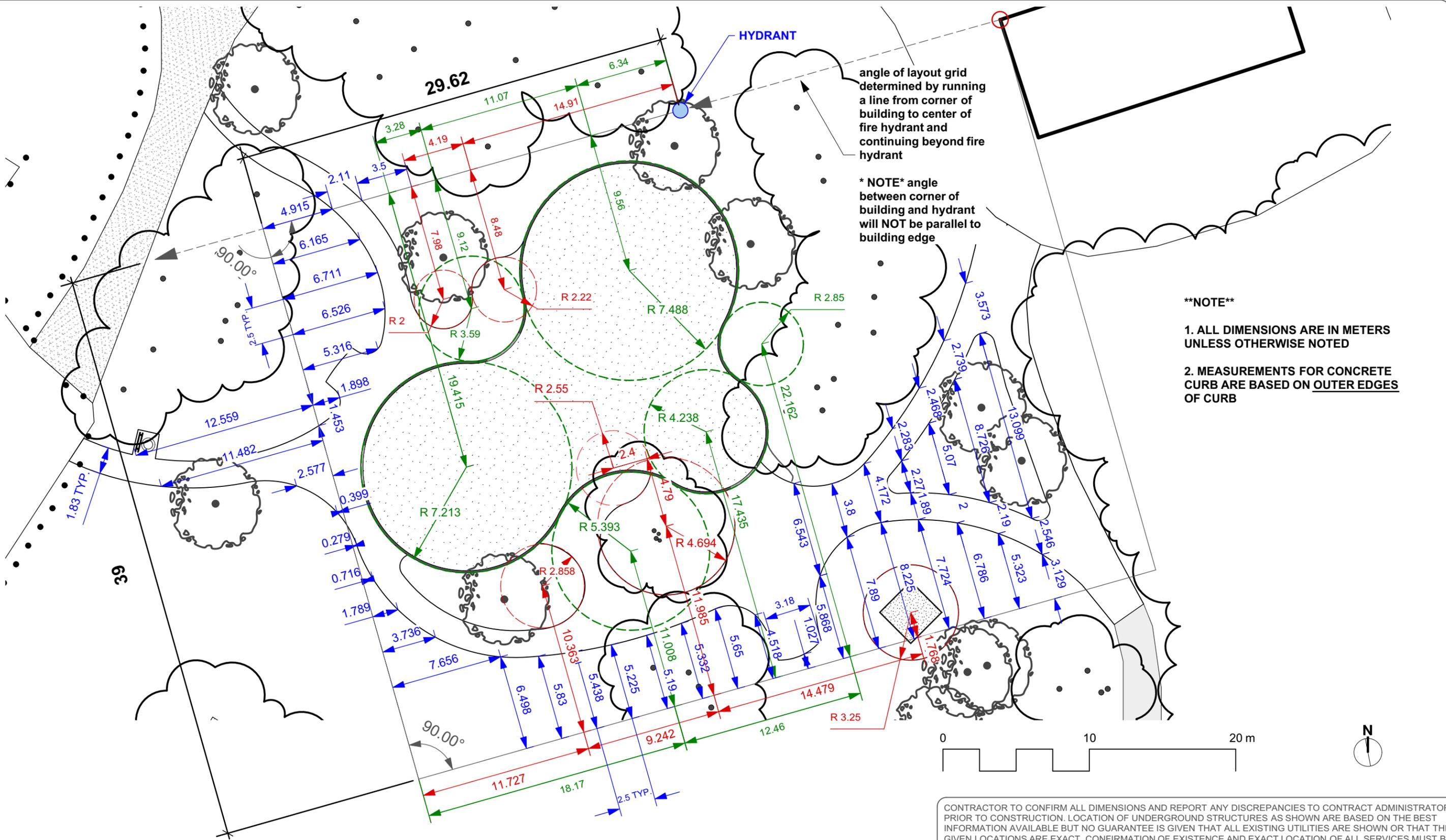
angle of layout grid determined by running a line from corner of building to center of fire hydrant and continuing beyond fire hydrant
