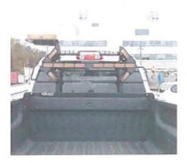
Directional Arrows and beacon/strobe for increased visibility, used as a blocking/shadowing vehicle
