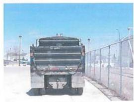
Beacon centered on lip of box with protective cage (recommended), providing 360° visibility in combination with strobe lights amber and blue on rear of vehicle (blue - snow removal operations only)
