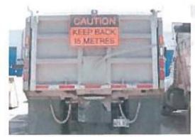
Amber Strobe light at top, with brake/signal/backup light array in side configuration
