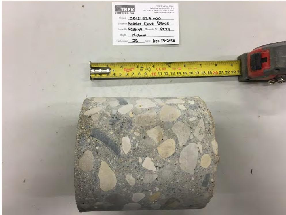
Photo 7: Pavement Core Sample at Test Hole PC18-44
