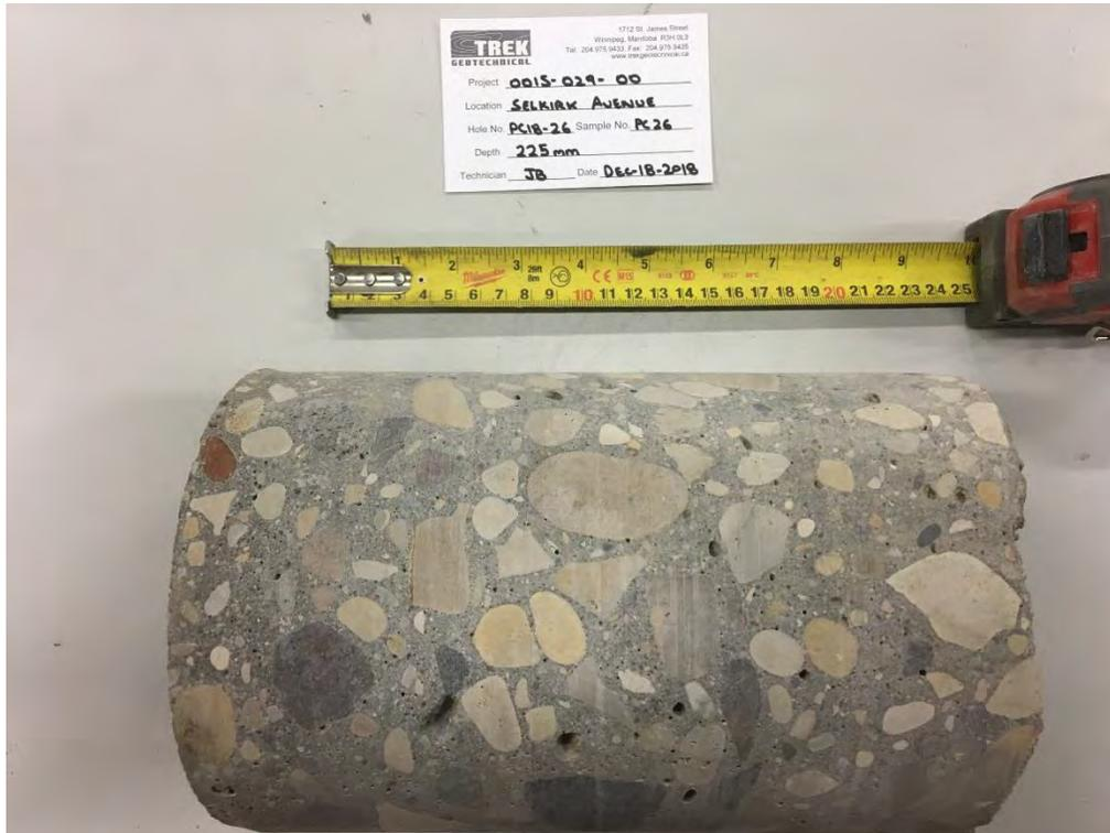
Photo 4: Pavement Core Sample at Test Hole PC18-26
