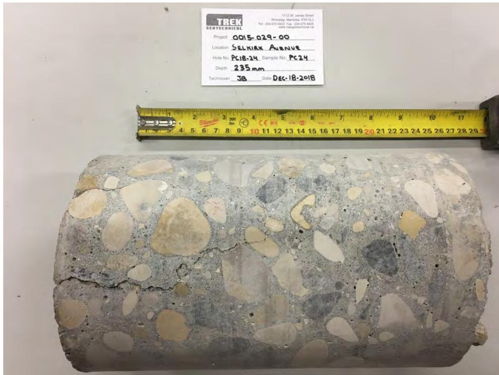
Photo 2: Pavement Core Sample at Test Hole PC18-24
