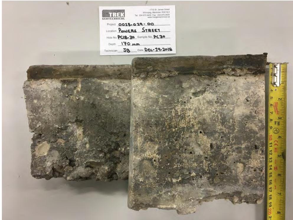
Photo 3: Pavement Core Sample view of Joint at Test Hole PC18-30
