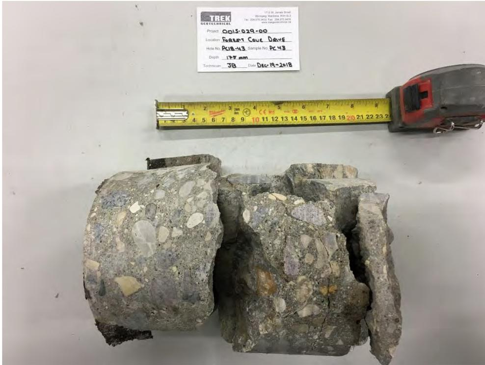
Photo 5: Pavement Core Sample at Test Hole PC18-43 (On Joint)
