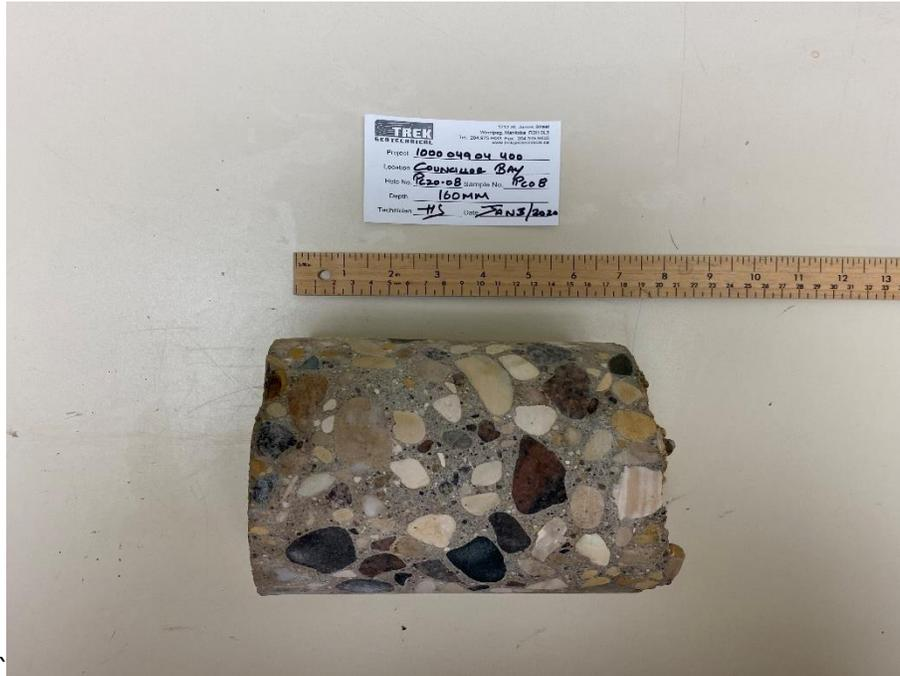
Photo 3: Pavement Core Sample at Pavement Hole PC20-08
