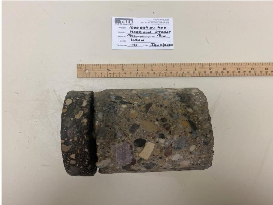
Photo 1: Pavement Core Sample at Pavement Hole PC20-01
