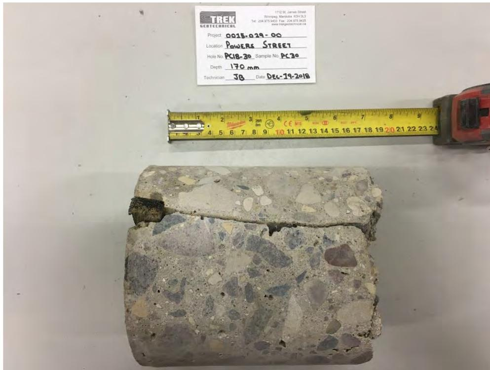
Photo 2: Pavement Core Sample at Test Hole PC18-30 (On Joint)
