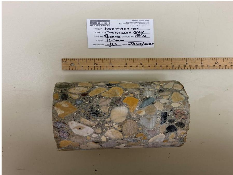
Photo 5: Pavement Core Sample at Pavement Hole PC20-10
