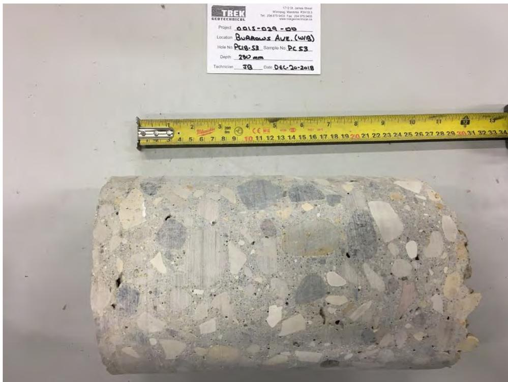
Photo 8: Pavement Core Sample at Test Hole PC18-53
