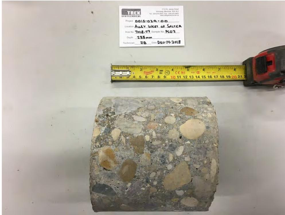
Photo 1: Pavement Core Sample at Test Hole TH18-07
