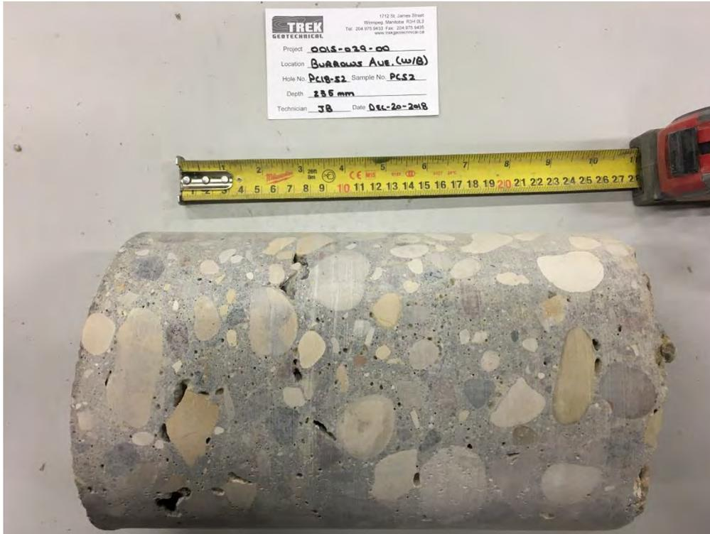
Photo 7: Pavement Core Sample at Test Hole PC18-52
