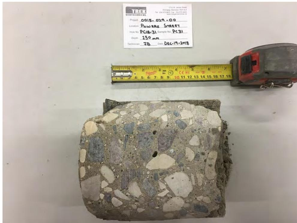
Photo 4: Pavement Core Sample at Test Hole PC18-31 (On Joint)
