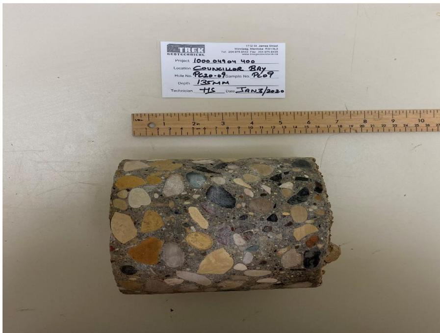
Photo 4: Pavement Core Sample at Pavement Hole PC20-09
