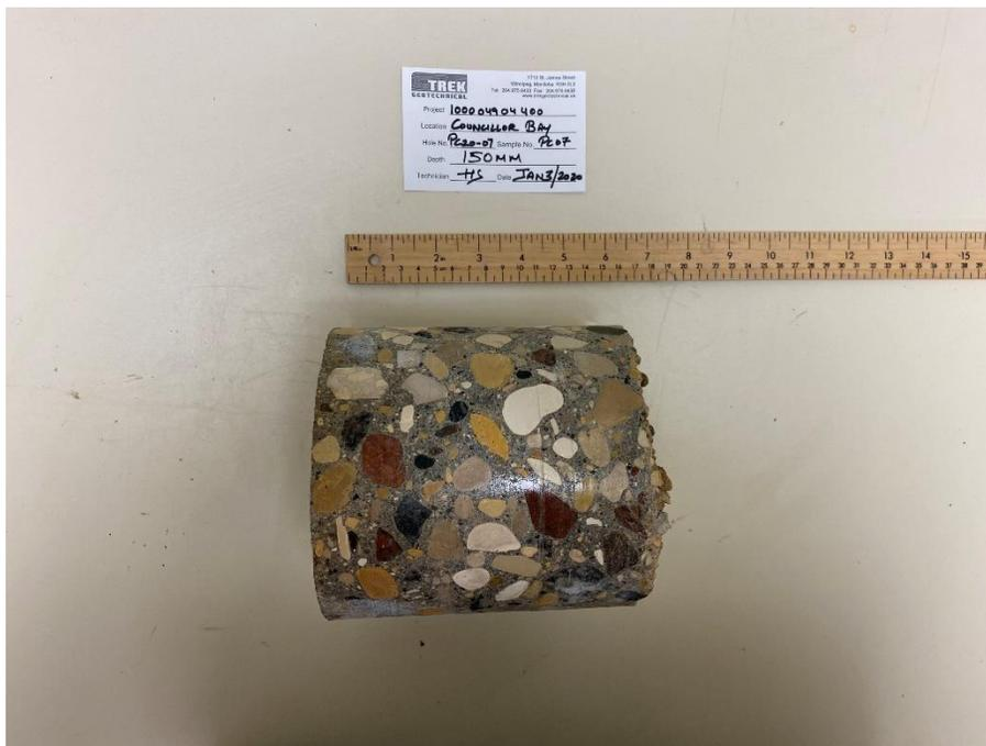
Photo 2: Pavement Core Sample at Pavement Hole PC20-07
