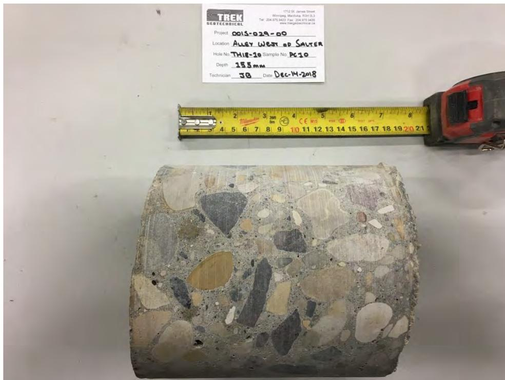
Photo 4: Pavement Core Sample at Test Hole TH18-10
