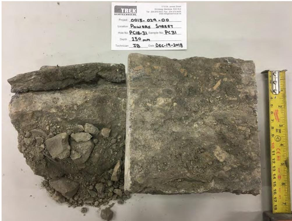
Photo 5: Pavement Core Sample view of Joint at Test Hole PC18-31
