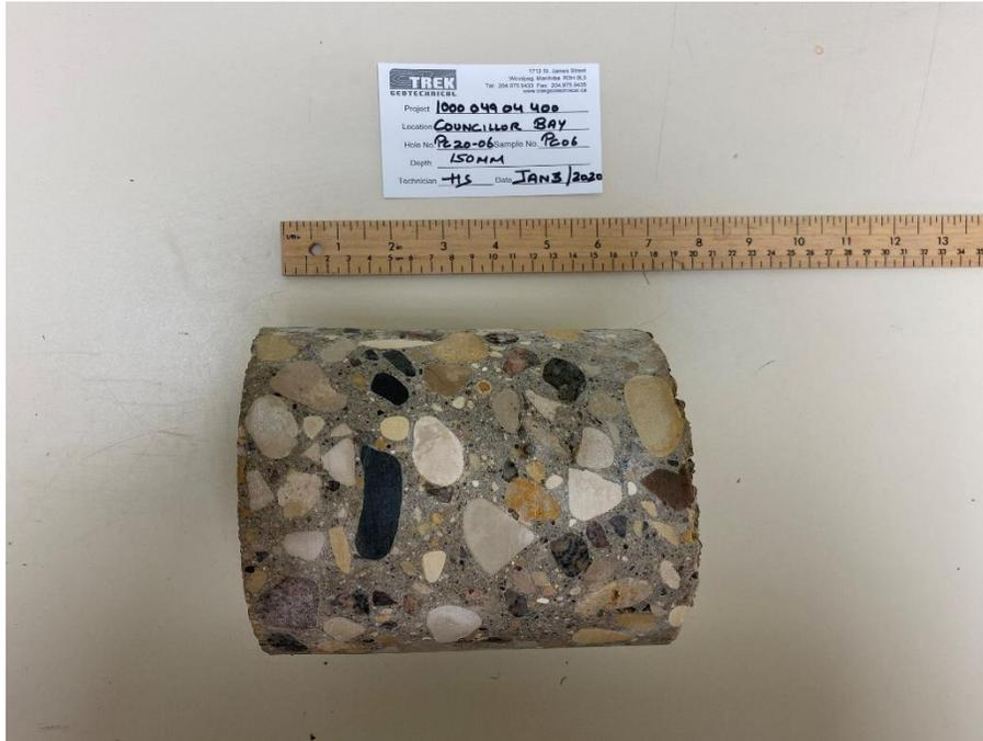
Photo 1: Pavement Core Sample at Pavement Hole PC20-06
