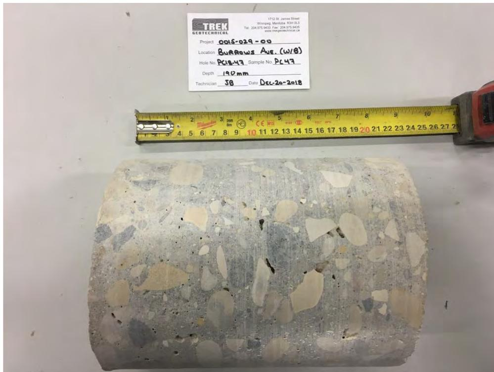
Photo 2: Pavement Core Sample at Test Hole PC18-47
