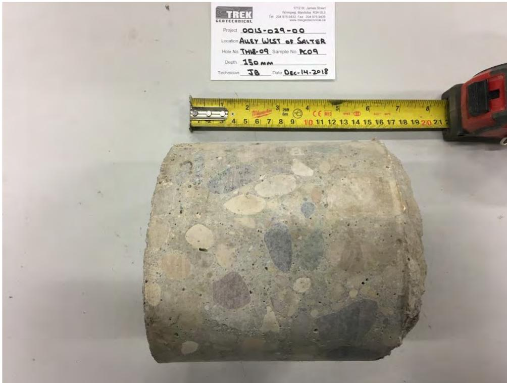
Photo 3: Pavement Core Sample at Test Hole TH18-09
