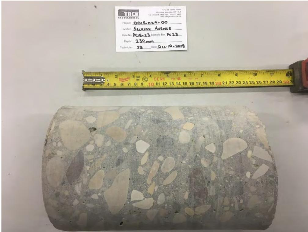
Photo 1: Pavement Core Sample at Test Hole PC18-23
