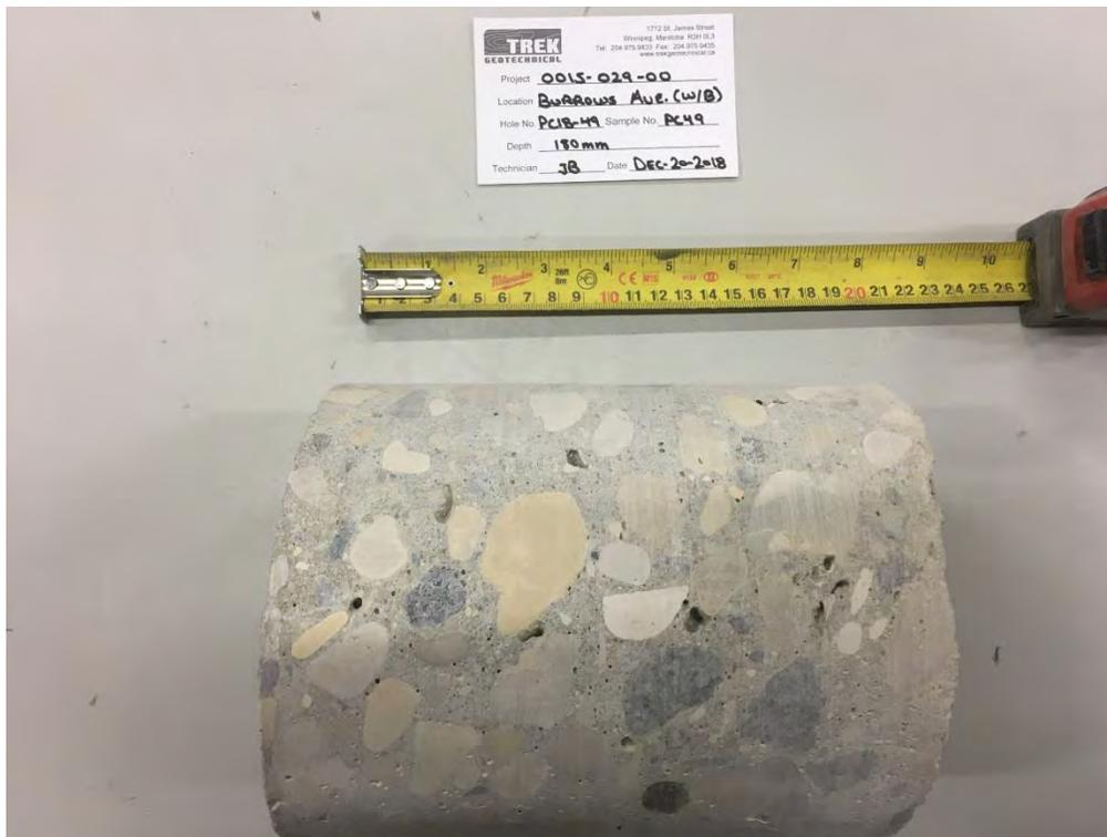
Photo 4: Pavement Core Sample at Test Hole PC18-49
