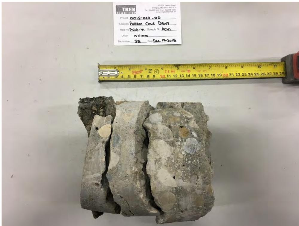
Photo 2: Pavement Core Sample at Test Hole PC18-41
