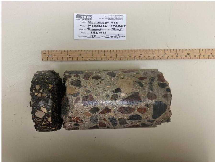
Photo 5: Pavement Core Sample at Pavement Hole 20-05
