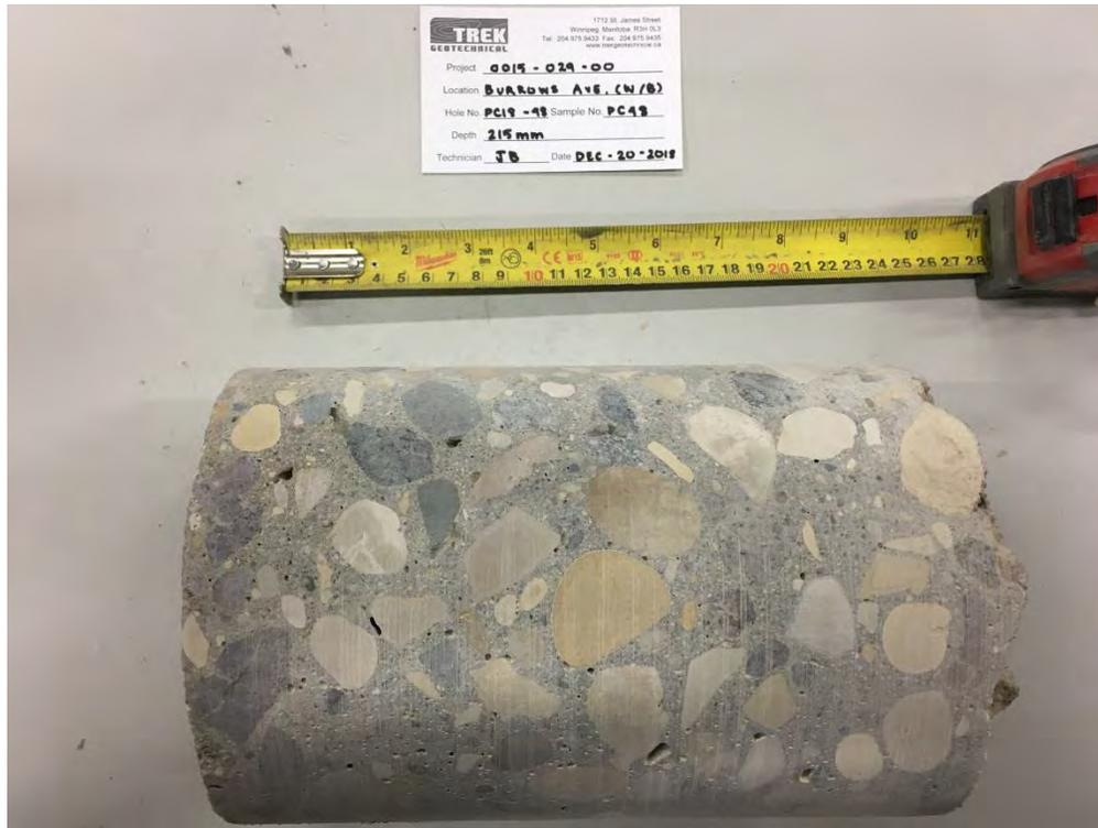
Photo 3: Pavement Core Sample at Test Hole PC18-48
