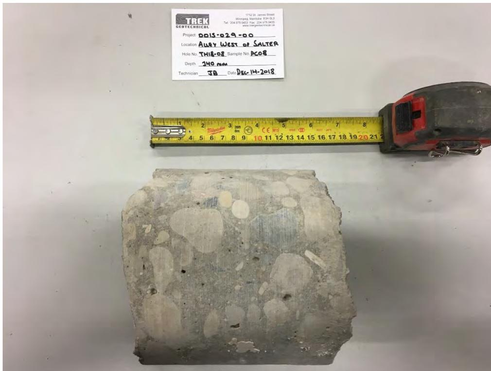
Photo 2: Pavement Core Sample at Test Hole TH18-08
