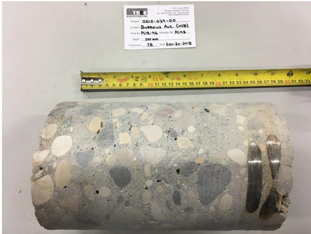
Photo 1: Pavement Core Sample at Test Hole PC18-46
