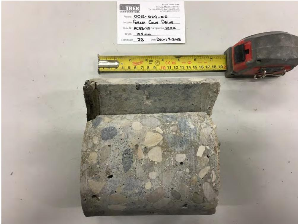
Photo 3: Pavement Core Sample at Test Hole PC18-42 (On Joint)
