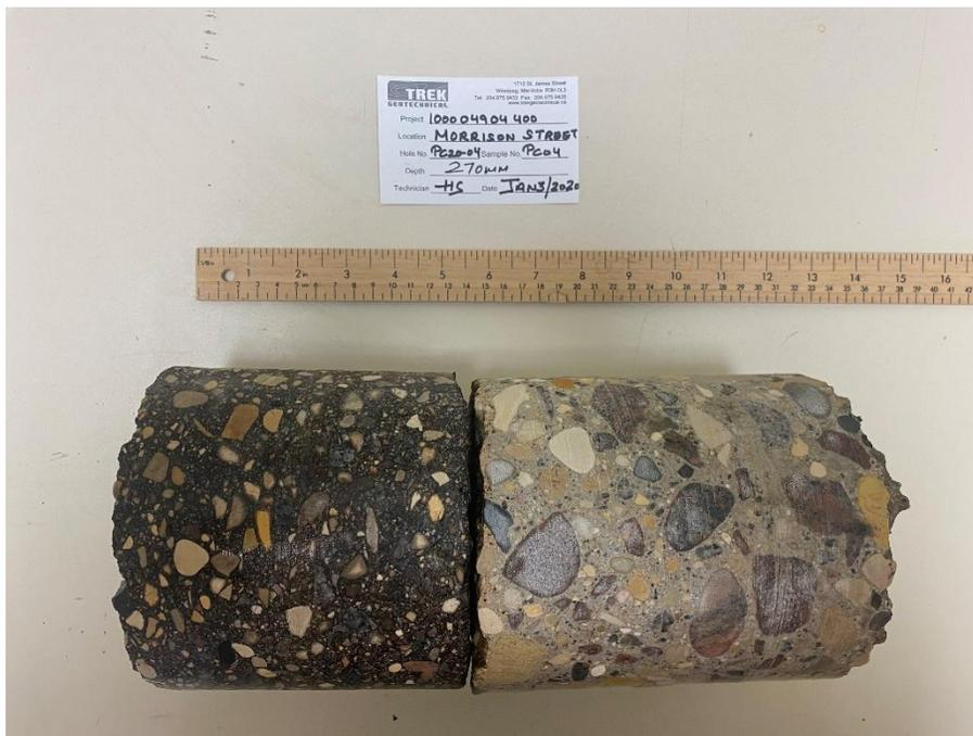
Photo 4: Pavement Core Sample at Pavement Hole PC20-04
