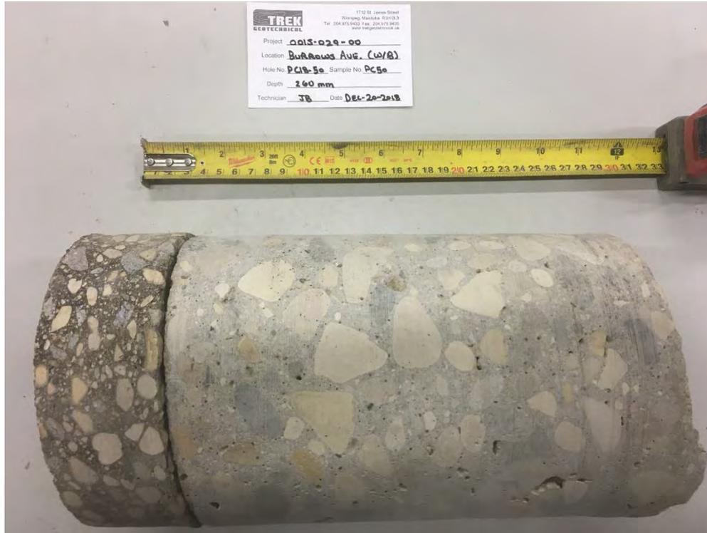
Photo 5: Pavement Core Sample at Test Hole PC18-50
