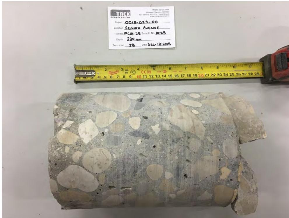
Photo 3: Pavement Core Sample at Test Hole PC18-25
