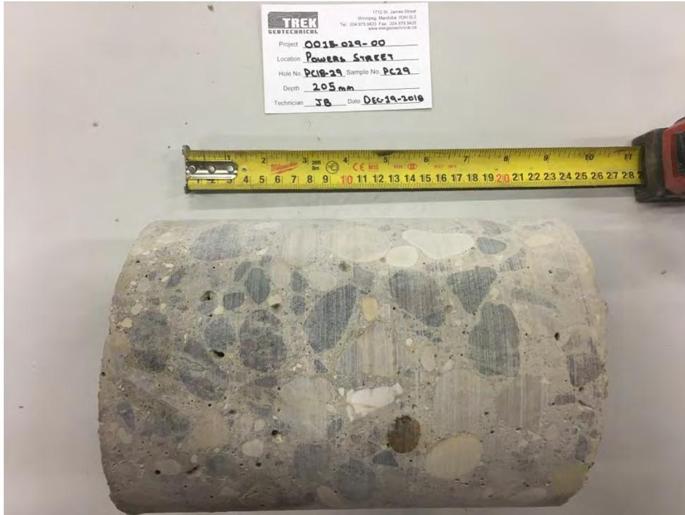
Photo 1: Pavement Core Sample at Test Hole PC18-29
