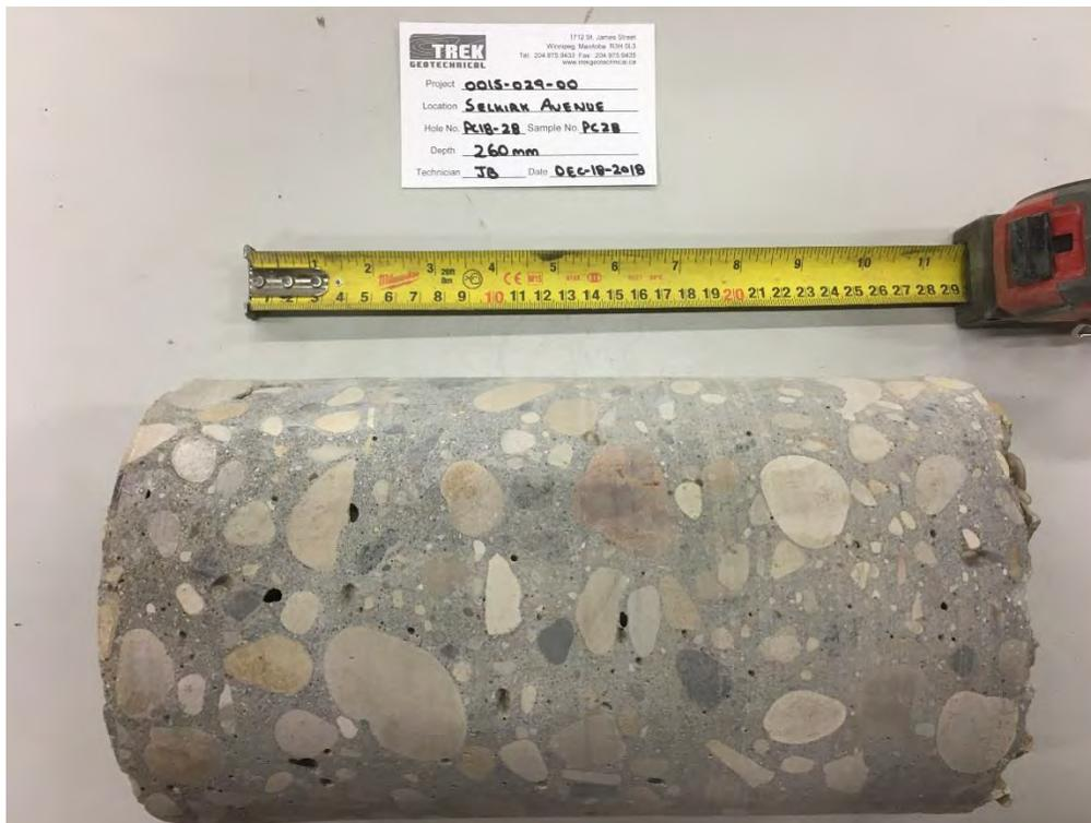
Photo 6: Pavement Core Sample at Test Hole PC18-28
