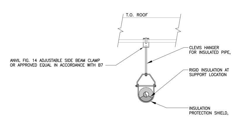
DETAIL - DRAIN WATER PIPE HANGER SUPPORT (TYP.) 0650M-M0002 <sub>SCALE: N.T.S.</sub>
