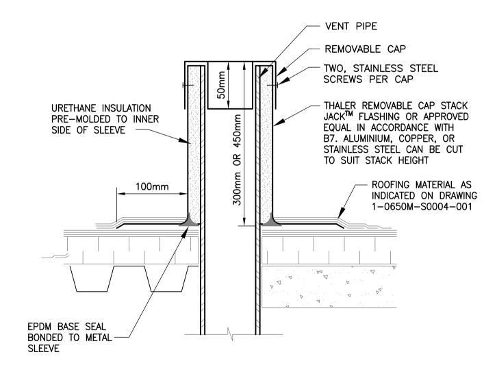
DETAIL - TYPICAL ROOF VENT 0650M-M0005 SCALE: N.T.S.
