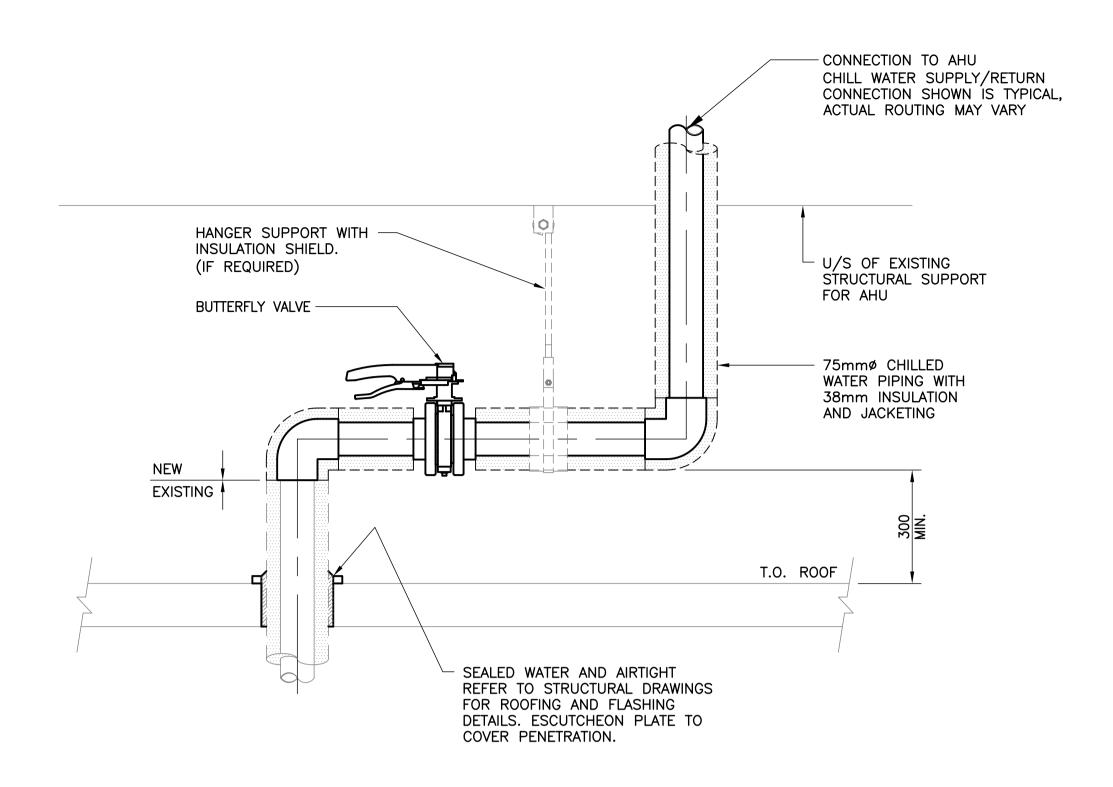
DETAIL - CHILLED WATER PIPING SUPPORT & CONNECTION 0650M-M0005 SCALE: N.T.S.
