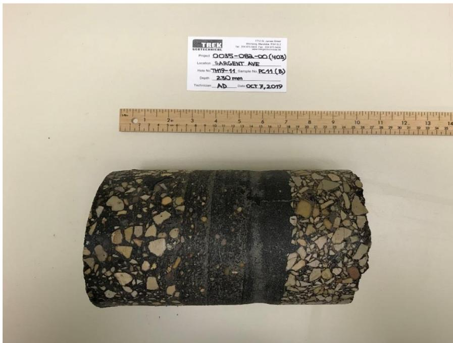
Photo 12: Pavement Core Sample at Test Hole TH19-11B
