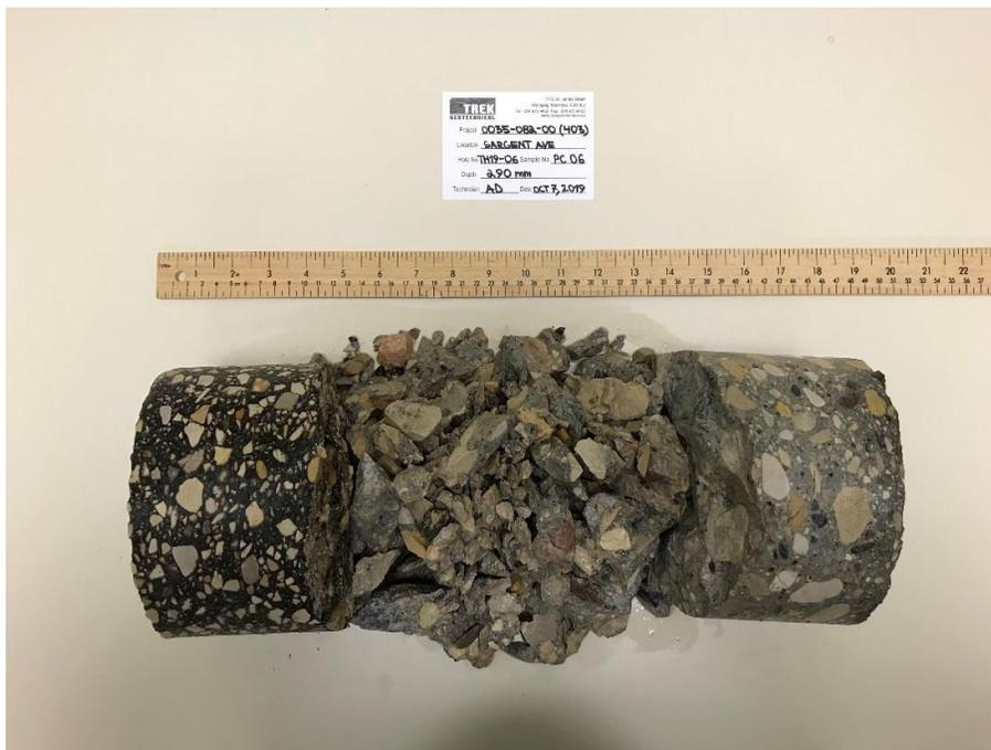
Photo 6: Pavement Core Sample at Test Hole TH19-06
