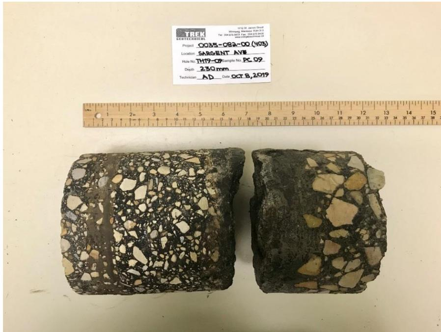
Photo 9: Pavement Core Sample at Test Hole TH19-09
