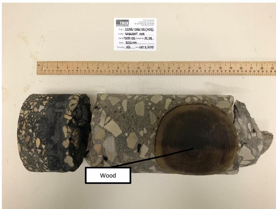
Photo 8: Pavement Core Sample at Test Hole TH19-08
