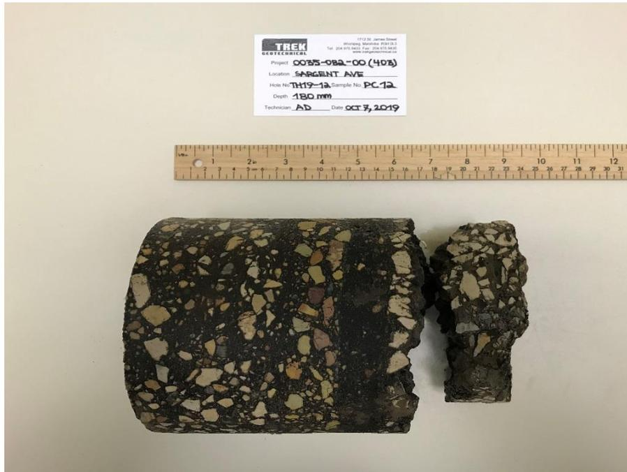
Photo 13: Pavement Core Sample at Test Hole TH19-12
