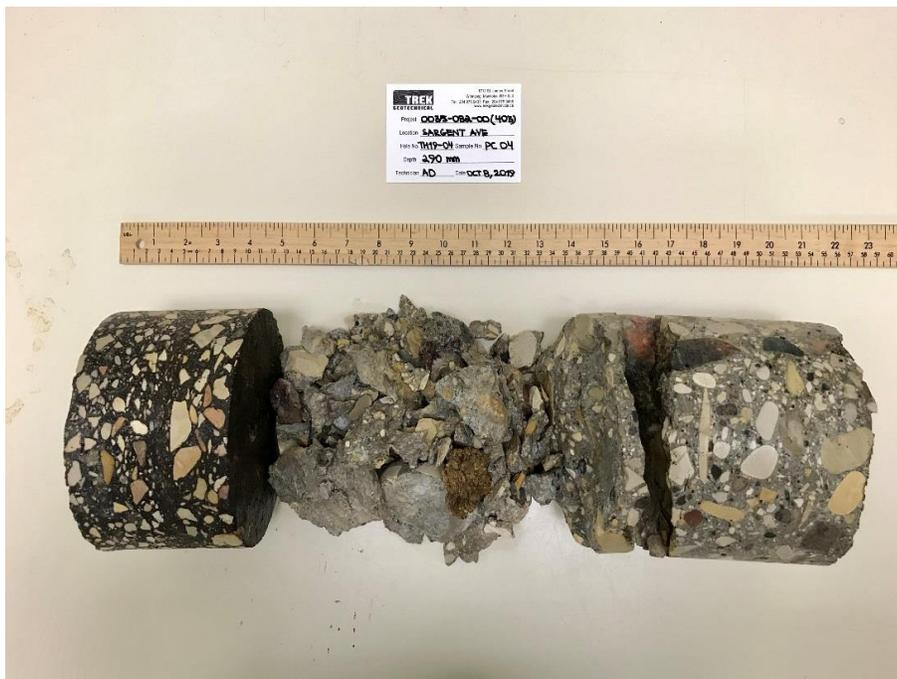
Photo 4: Pavement Core Sample at Test Hole TH19-04
