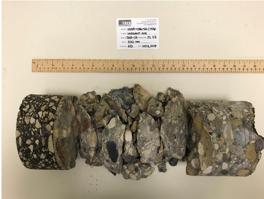
Photo 3: Pavement Core Sample at Test Hole TH19-03
