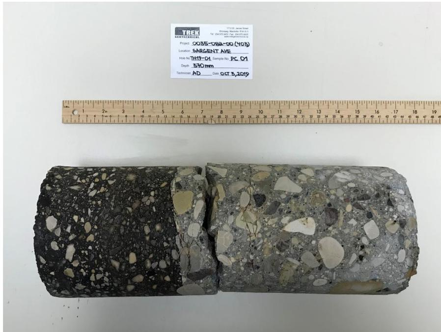
Photo 1: Pavement Core Sample at Test Hole TH19-01
