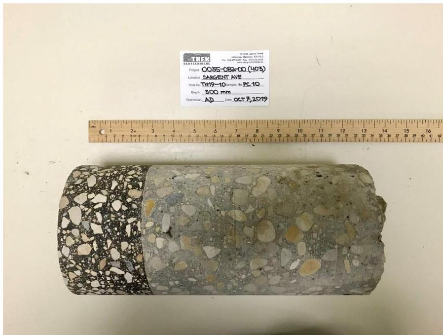
Photo 10: Pavement Core Sample at Test Hole TH19-10
