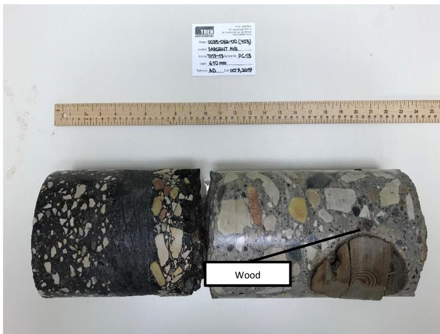
Photo 14: Pavement Core Sample at Test Hole TH19-13
