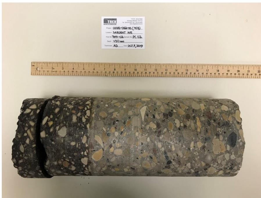
Photo 2: Pavement Core Sample at Test Hole TH19-02
