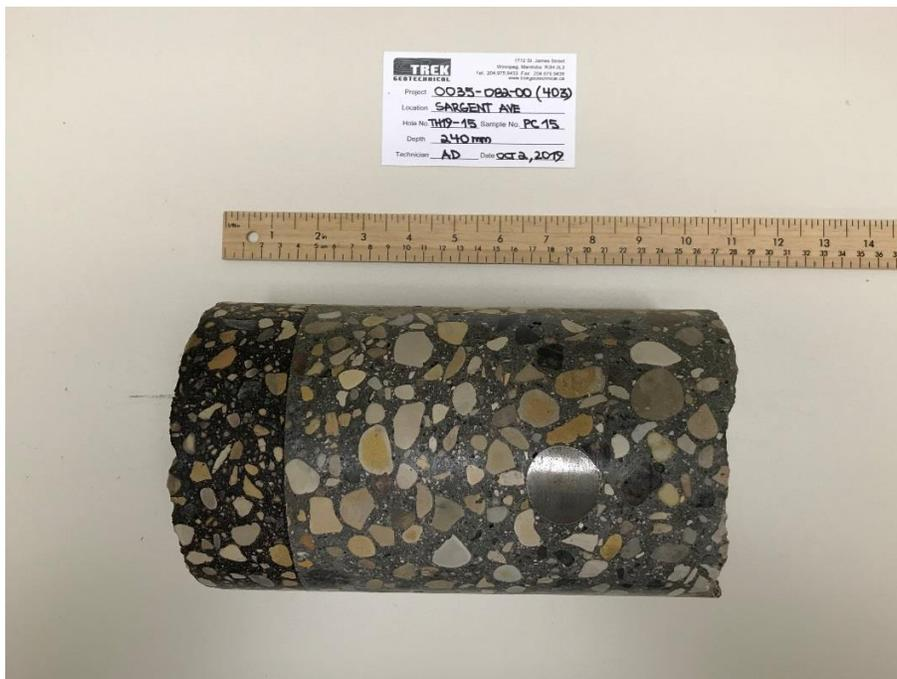
Photo 16: Pavement Core Sample at Test Hole TH19-15
