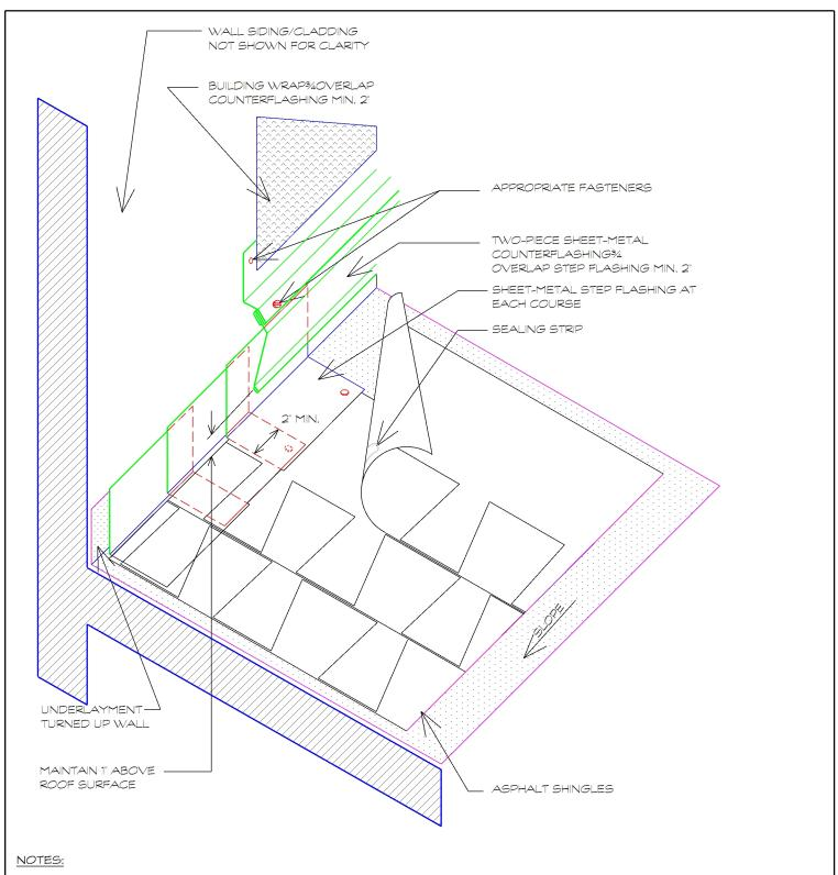
FOR SECUREMENT AND JOINERY OPTIONS FOR SHEET METAL AND COUNTERPLASHING OPTIONS, REFER TO THE CRCA ROOFING MANUAL.
