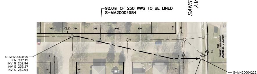
SEWER JUNCTION INFORMATION FROM SEWER VIDEO INSPECTION SEWER ID S-MA20004584 DISTANCE FROM MH ID S-MH20004199 DISTANCE DIAMETER CLOCK 200 15.1 200 11 28.0 200 10 47.0 200 10 47.6 200 10 \*\*\*\*REVERSAL REQUIRED\*\*\*\*
