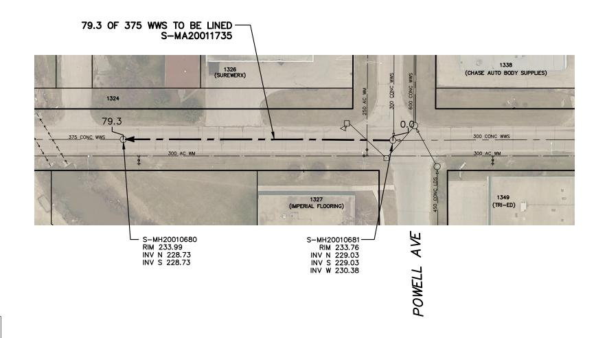
SEWER JUNCTION INFORMATION FROM SEWER VIDEO INSPECTION SEWER ID S-MA20011735 DISTANCE FROM MH ID S-MH20010681
