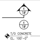
SECTION MARKER (MEANS SECTION X SHOWN ON DRAWING SHEET S#)
