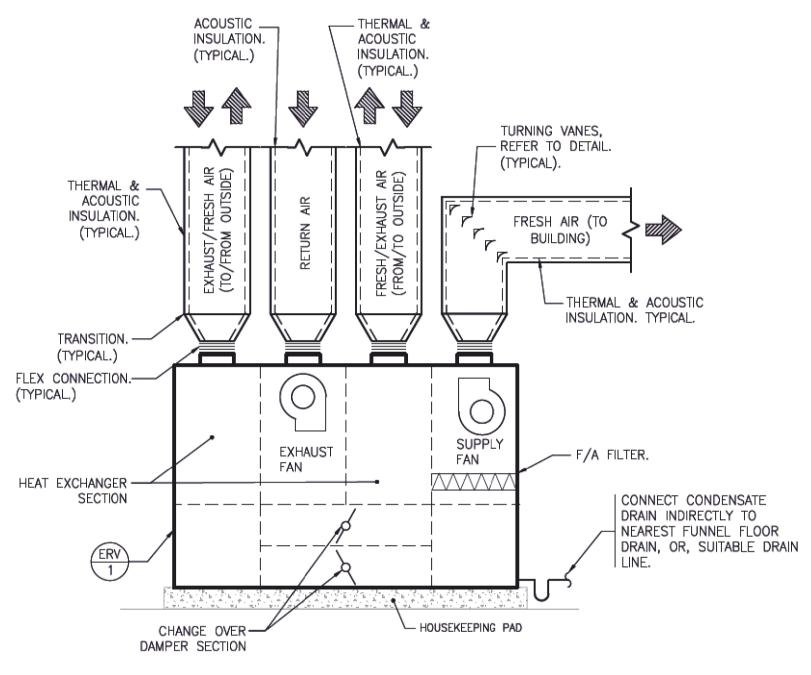
**ENERGY RECOVERY** VENTILATOR/DOAS (ERV-1) DETAIL SCALE: N.T.S.
