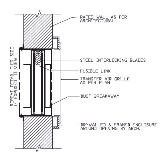
FIRE DAMPER TO BE INSTALLED AS PER MANUFACTURER'S RECOMMENDATION. DUCT/COLLAR BREAKAWAY CONNECTION TO BE APPROVED.
