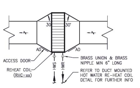
DUCT MOUNTED HEATING RE-HEAT COIL ACCESS (TYPICAL)
