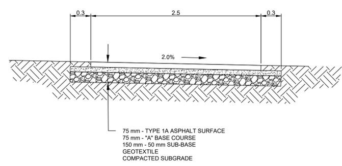
**75 mm ASPHALT PATH TYPICAL CROSS SECTION**
