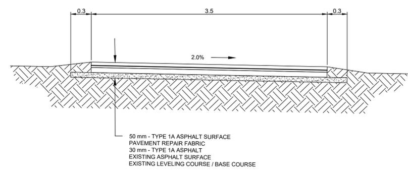
**B** 75 mm ASPHALT PATH CROSS SECTION
