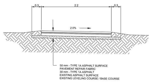
**A** 75 mm ASPHALT PATH CROSS SECTION
