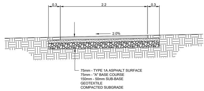
**75 mm ASPHALT PATH TYPICAL CROSS SECTION**
