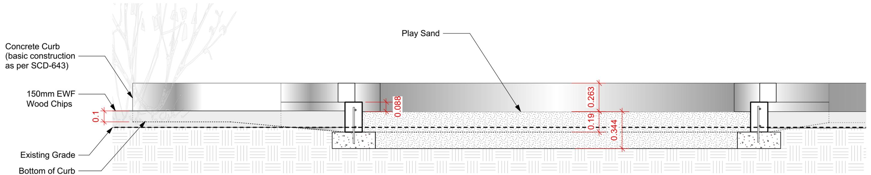
**5 Sand Box and Concrete Edging Cross Section 1**
