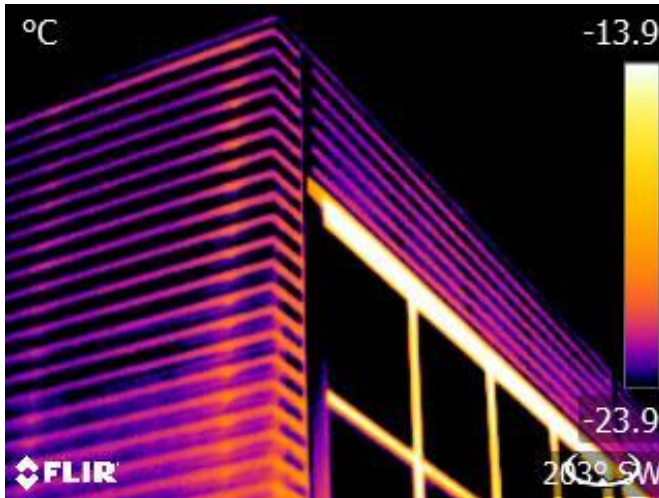
Figure 6: Thermal bridge at window frames at North elevation (refer to Photograph #65).
