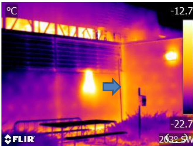
Figure 7: Thermal bridge at inside corner of North elevation wall intersection at entrance (refer to Photograph #5). Direct path for heat flow from mass of masonry at the corner causes elevated temperatures on the exterior surface during colder weather.
