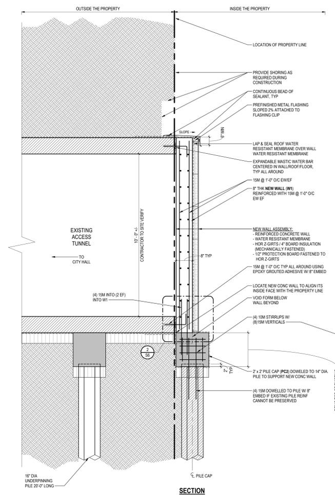
**1 SECTION DETAIL @ TUNNEL END CAP**
