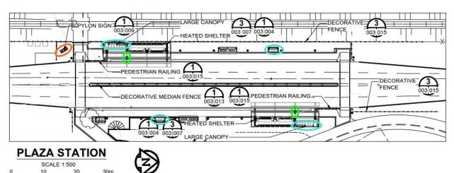
Figure 18: Plan View of Signs at Plaza Station
