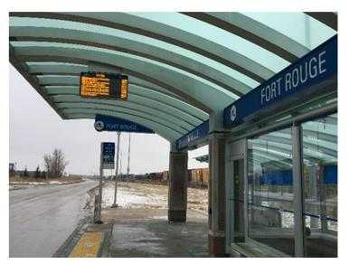
Figure 5: Type C BUSwatch Sign Suspended From Platform Canopy at Fort Rouge Station
