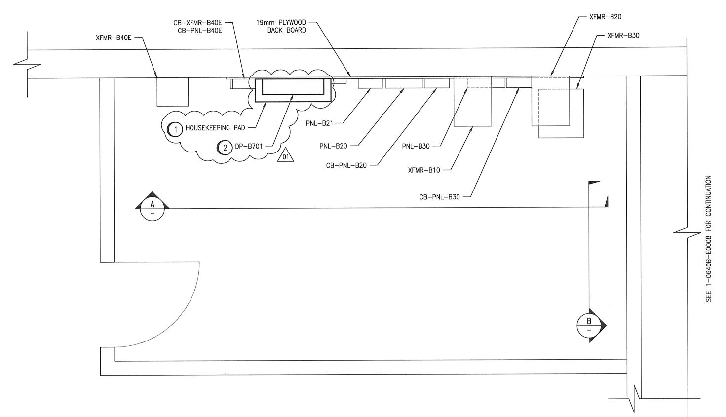
ELECTRICAL ROOM: ELECTRICAL PLAN LAYOUT SCALE: 1 : 20
