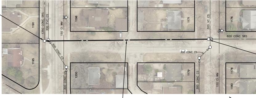
V GROSVENOR L105.3 OF 600 CONC SRS TO BE LINED S-MA60021439 (PARTIALLY DETERIORATED)
