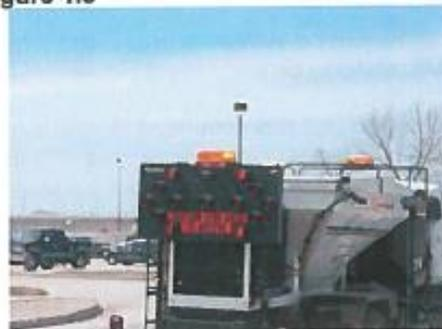
Figure 1.2 and 1.3: Roadpatcher with directional lighting and informational sign (note front and rear mounted beacon lights)
