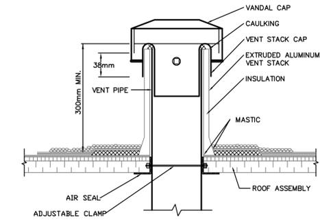
2 TYPICAL VENT THROUGH ROOF DETAIL
