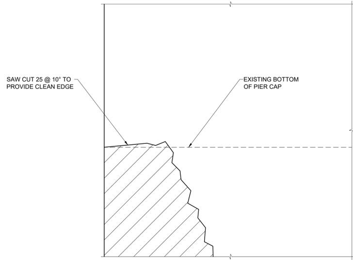
**6** **DETAIL - CONCRETE REMOVALS FOR CHAMFER**
