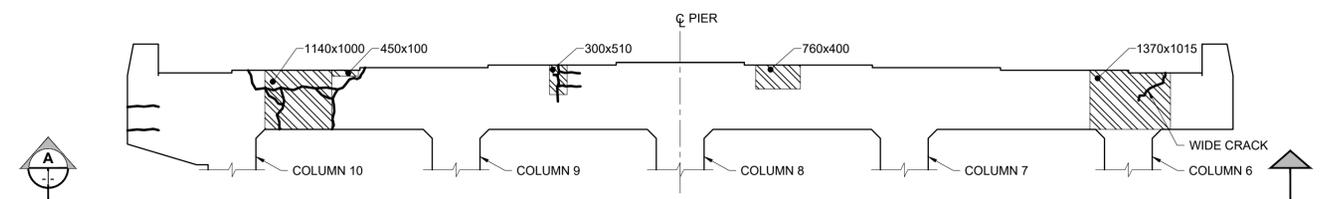
**CENTRE PIER CAP ELEVATION - NORTH FACE**
