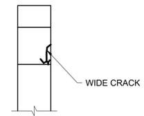
**CENTRE PIER CAP WEST END ELEVATION**
