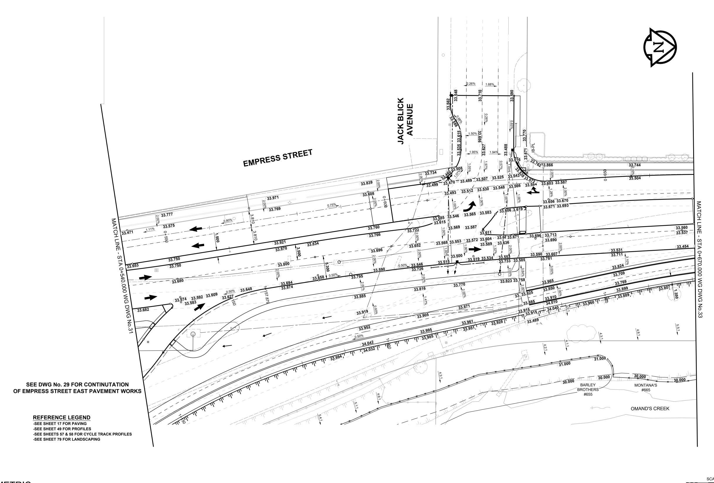
1. ADJUST MH'S,CB RIMS, WV'S AND HYD'S TO NEW GRADES. 2. CONTRACTOR TO REGRADE/RENEW EXST PRIVATE SIDEWALKS TO LIMITS AS SHOWN. SIDEWALKS TO BE RENEWED WITH CONCRETE UNLESS NOTED OTHERWISE.
