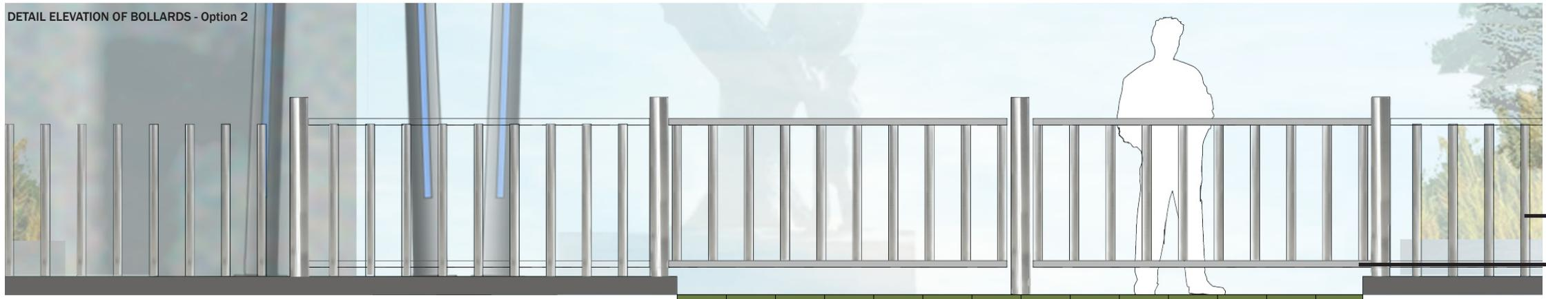
Stainless steel bollards on raised concrete curb
