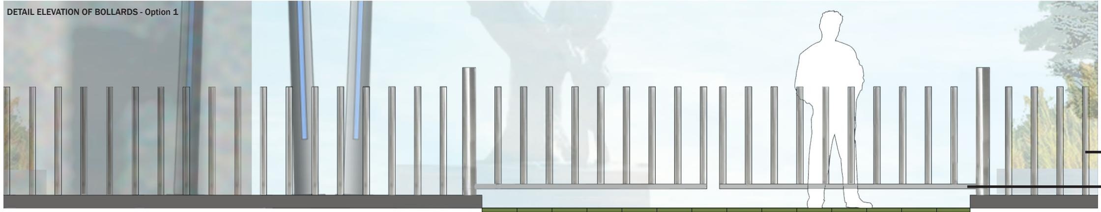
Stainless steel bollards on raised concrete curb
