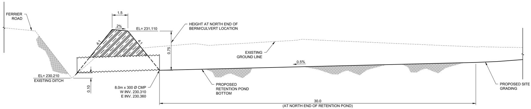
**E-E** 1.5 m WIDE PERIMETER BERM/CULVERT DETAIL – ALONG FERRIER ROAD
