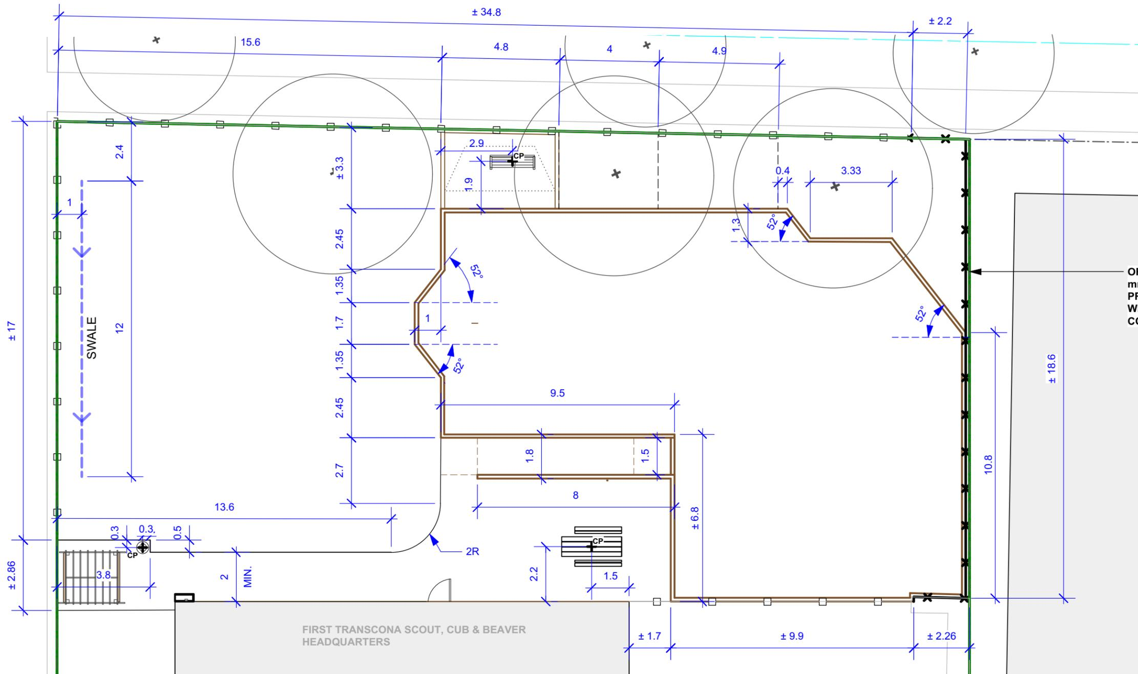
OFFSET NEW 1.5 m CHAINLINK FENCE 150 mm FROM PROPERTY LINE. CONFIRM PROPERTY SURVEY PINS WITH CITY OF WINNIPEG GEOMATICS BRANCH PRIOR TO CONSTRUCTION.
