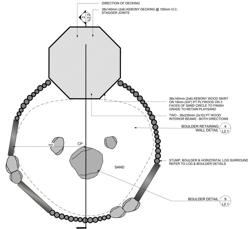
1 SAND CIRCLE & STAGE DECKING DETAIL PLAN
