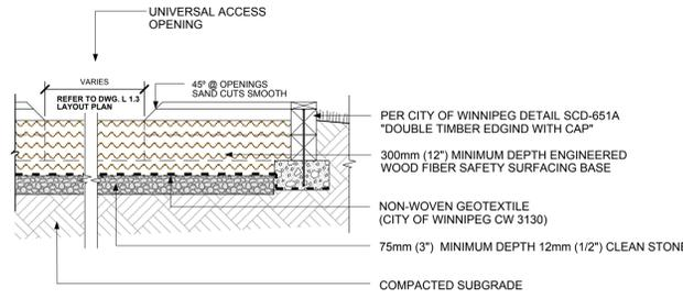
1 SAFETY SURFACING & WOOD TIMBER EDGE DETAIL
