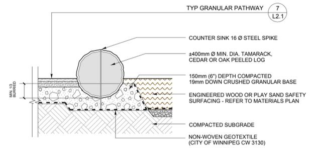
4 LOG RETAINING WALL DETAIL
