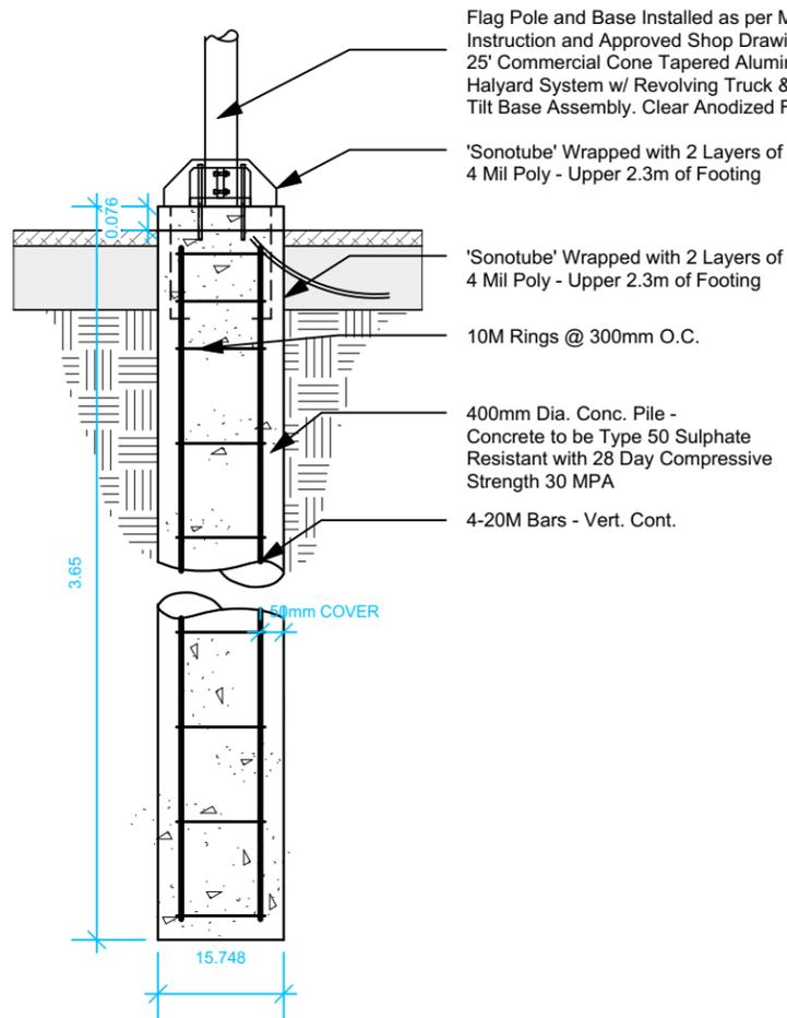
Flag Pole and Base Installed as per Manufacturer's Written Instruction and Approved Shop Drawings. Pole to be HTA25N - 25' Commercial Cone Tapered Aluminum Flagpole c/w Internal Halyard System w/ Revolving Truck & 6" Silver Ball Top. B-7 Tilt Base Assembly. Clear Anodized Finish.
