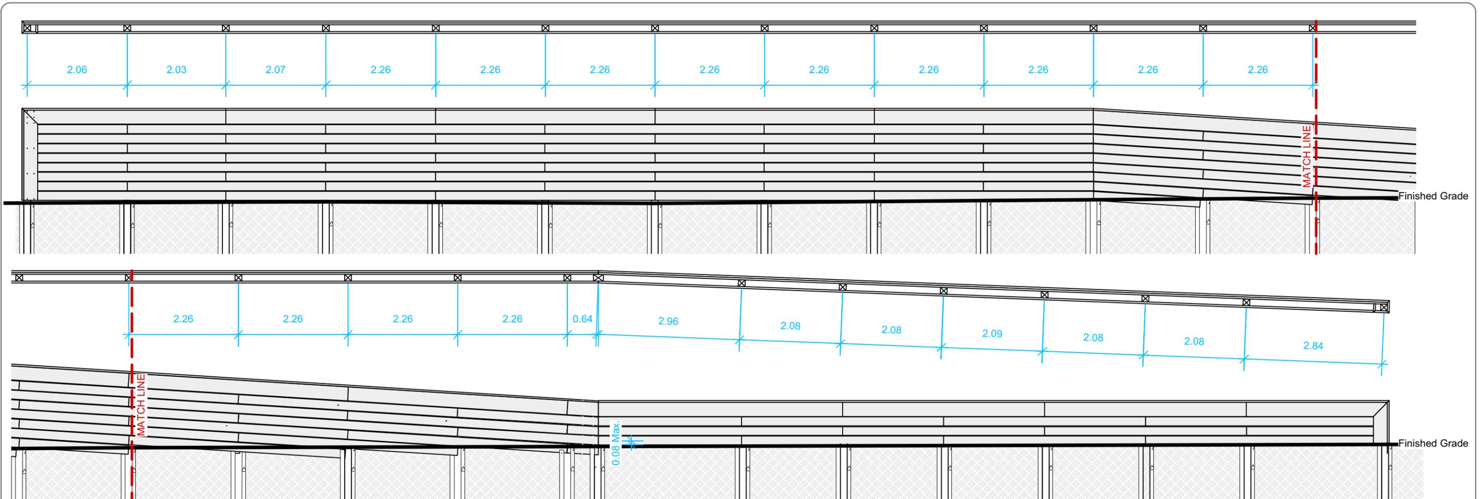
1 1.85M, ANGLED FENCE AND 1.27M FENCE ELEVATION
