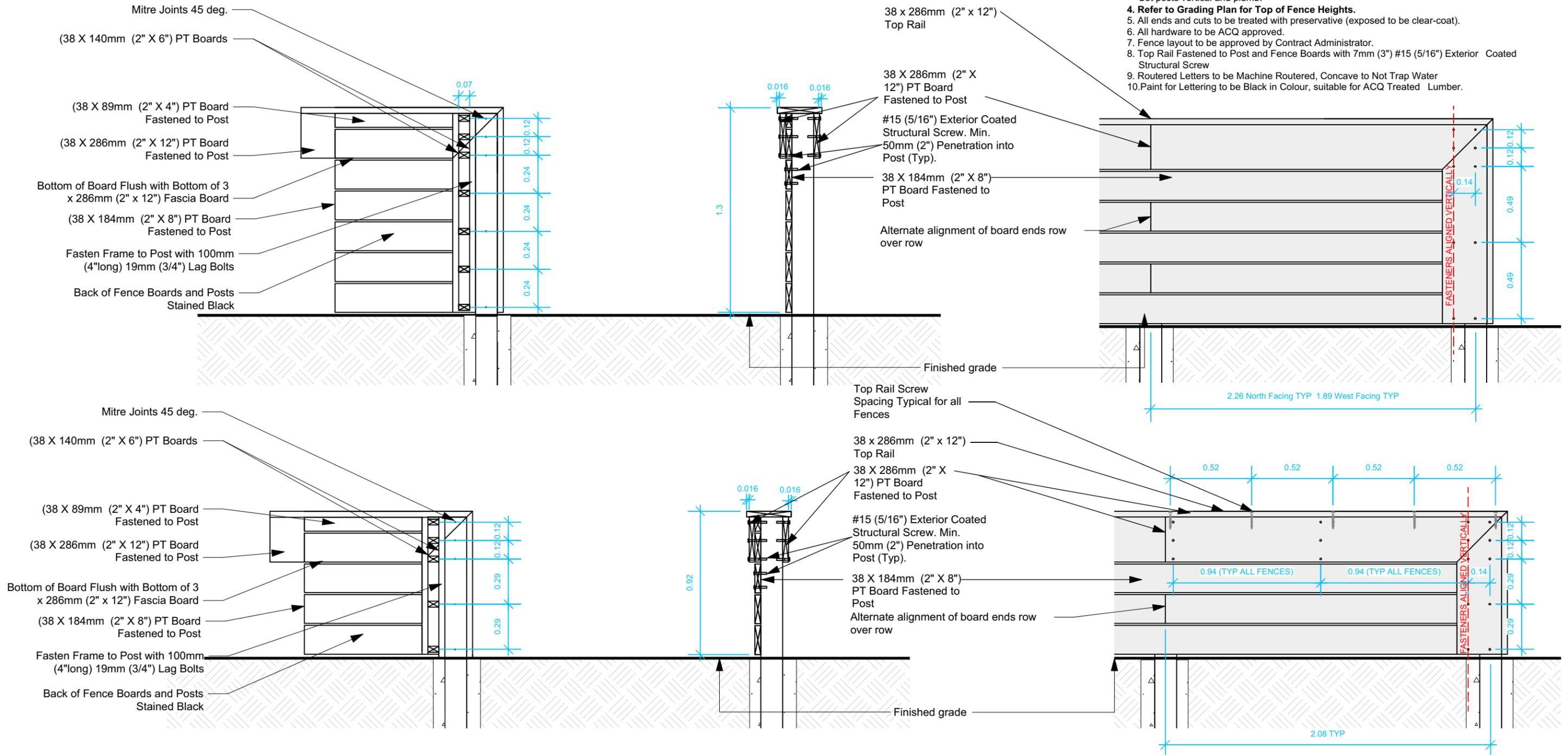
1 0.9M & 1.27M FENCE SECTIONS AND ELEVATIONS
