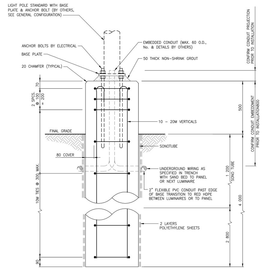
**POLE MOUNTED LUMINAIRE BASE DETAIL**
