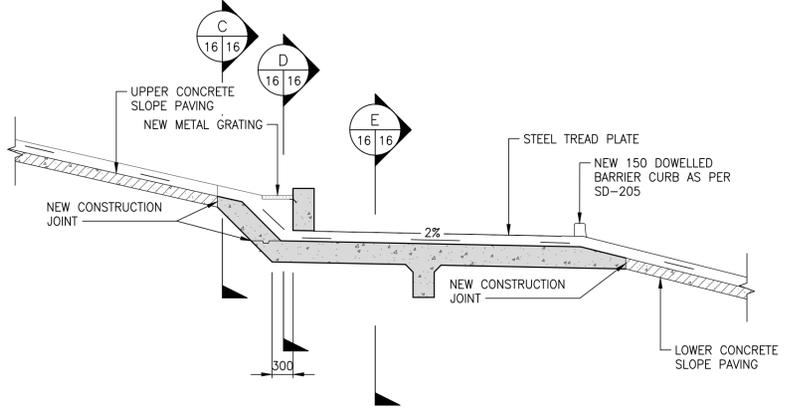
**PROPOSED SECTION THROUGH HEADSLOPE DRAIN**
