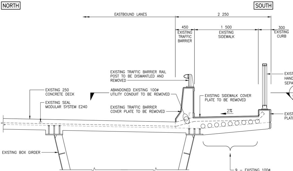
TYPICAL EXISTING ELEVATION AT ABUTMENT
