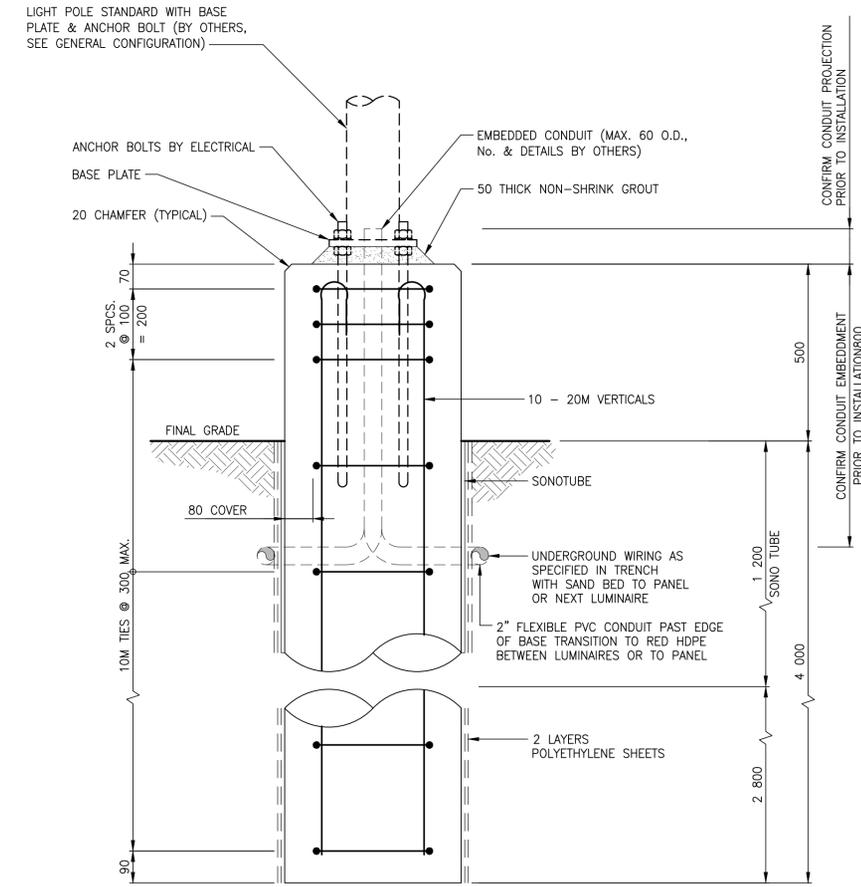
**POLE MOUNTED LUMINAIRE BASE DETAIL**
