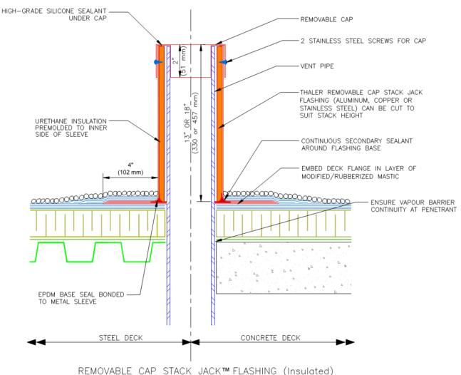
REMOVABLE CAP STACK JACK™ FLASHING (Insulated)
