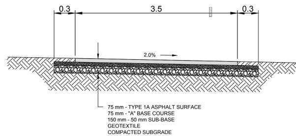
ASPHALT PATH TYPICAL CROSS SECTION
