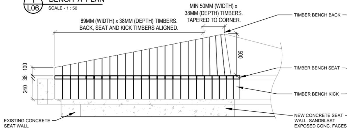
BENCH SUPPORT STEEL STRAPS. RUN FRONT TO BACK, ALIGNED WITH BACK, SEAT AND KICK. SPACED EQUALLY FROM BENCH ENDS TO CORNERS. MAX 1200MM SEPARATION. STRAPS CENTERED BEHIND TIMBERS. REFER TO L06/4
