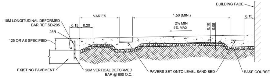
TYPICAL MONOLITHIC CURB AND SIDEWALK - SECTION VIEW
