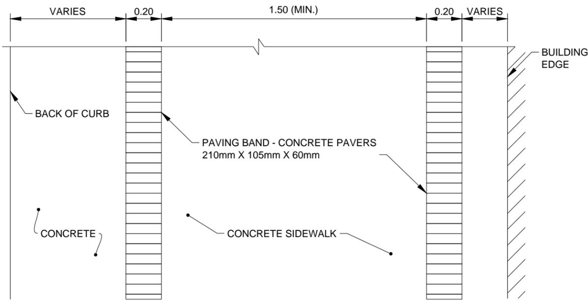
1 TYPICAL PAVING BAND PATTERN - PLAN VIEW
