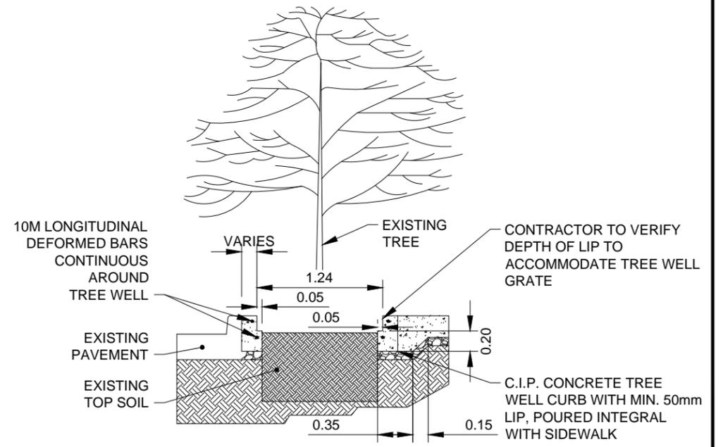
5 TYPICAL TREE WELL AT EXISTING TREE - SECTION VIEW
