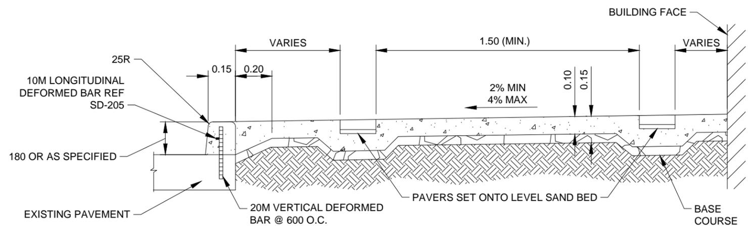
2 TYPICAL CURB & SIDEWALK - SECTION VIEW
