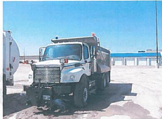
Double beacons mounted on lip of box with protective cage (recommended), providing 360° visibility (blue - snow removal operations only) – blue lens and/or beacon to be de-energized for all non snow removal operations
