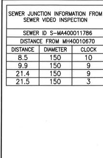
MH ID MH40010670 RIM 233.240 INV N 231.670 INV E 231.670 INV W 231.670 6.4 OF 200 SDR35 PVC SEWER REPAIR (SD-022B). INCLUDING 1 SERVICE
